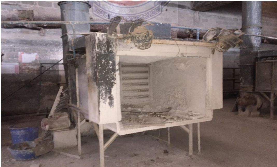
Fig 23: An image of a test kiln which was used in the industry
