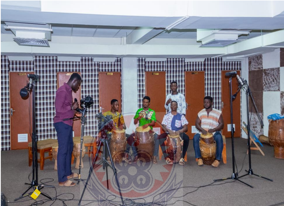
Figure 42: Spaced Pair Microphone Technique used to record instrumental patterns
