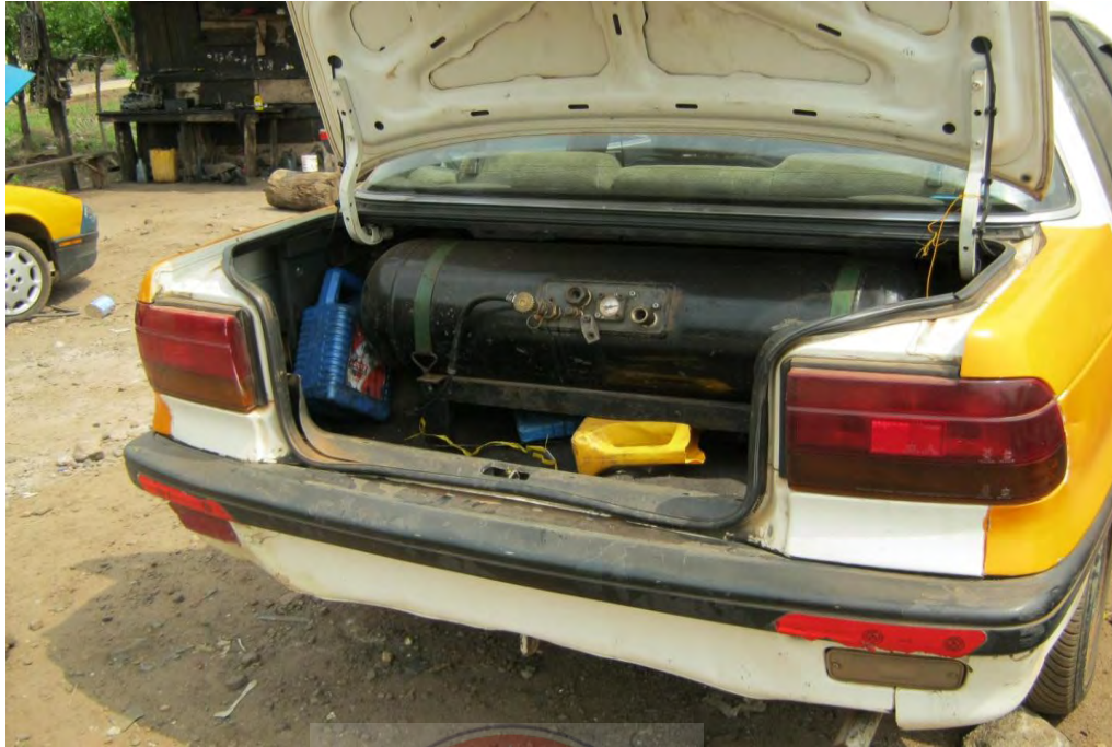
Figure 5.7. Transversal mounted Fuel Container, located in the boot of the automobile.
