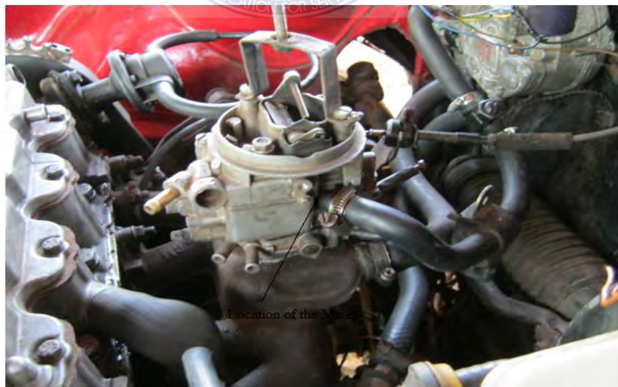
Figure 5.2. Mixer incorporated Carburettor, showing the location of the Mixer.
