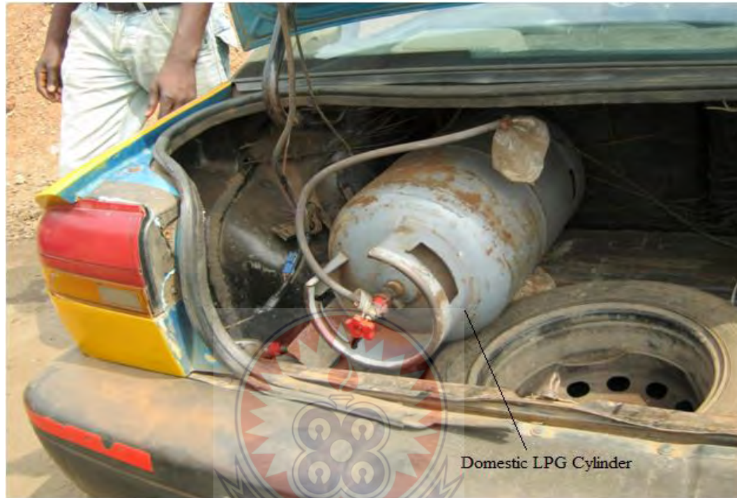
Figure 5.5. Unauthorized domestic cylinder usage as fuel container in automobile.
