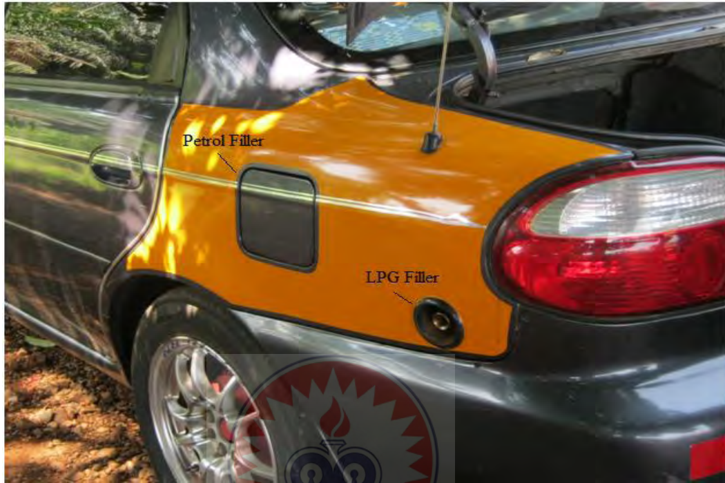
Figure 5.10. Ideal Filler locations for converted LPG and petrol alternative automobile.
