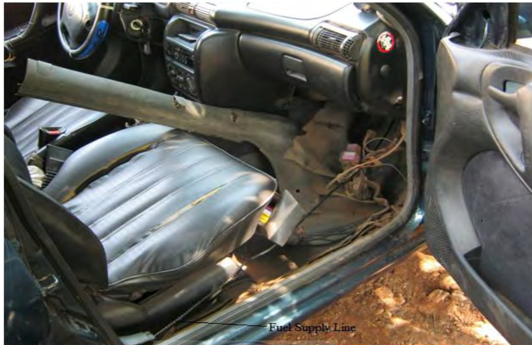
Figure 5.12. Fuel Line passed through inside vehicle at the passenger side of the automobile.
