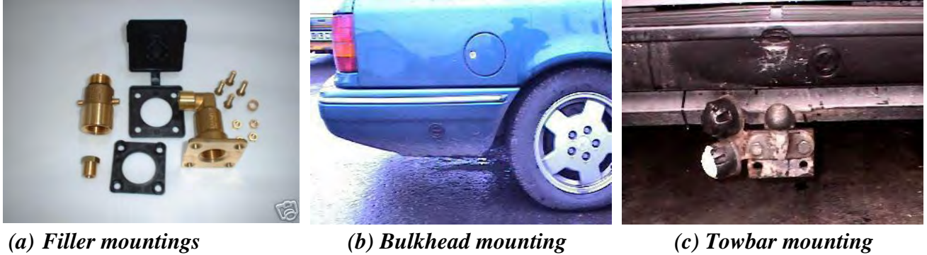
Figure 2.8. Options of filler mountings; (a) Filler mountings, (b) Bulkhead mounting, (c) Towbar mounting
