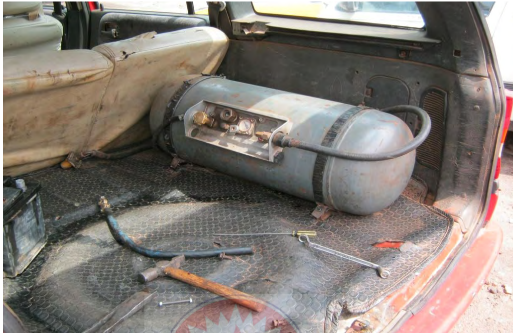
Figure 5.6. Unsafe longitudinal mounting of fuel container in the boot of automobile.
