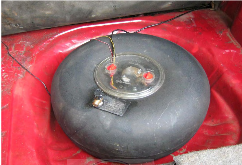
Figure 5.8. Toroidal Fuel Container; located in the spare wheel well with incomplete airtight box system.
