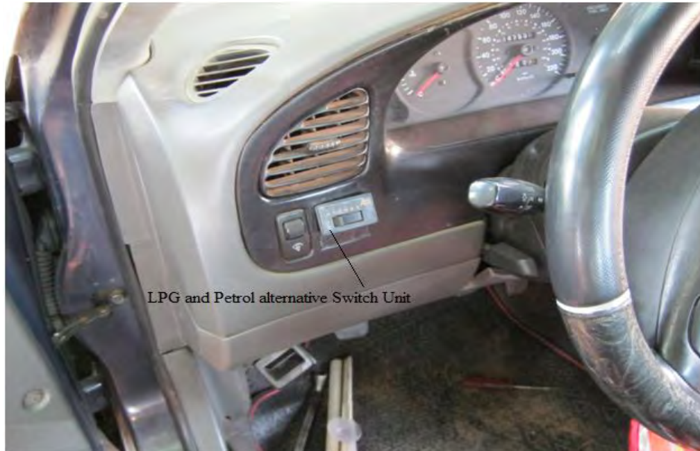
Figure 5.11. LPG and Petrol alternative Switch Unit location.
