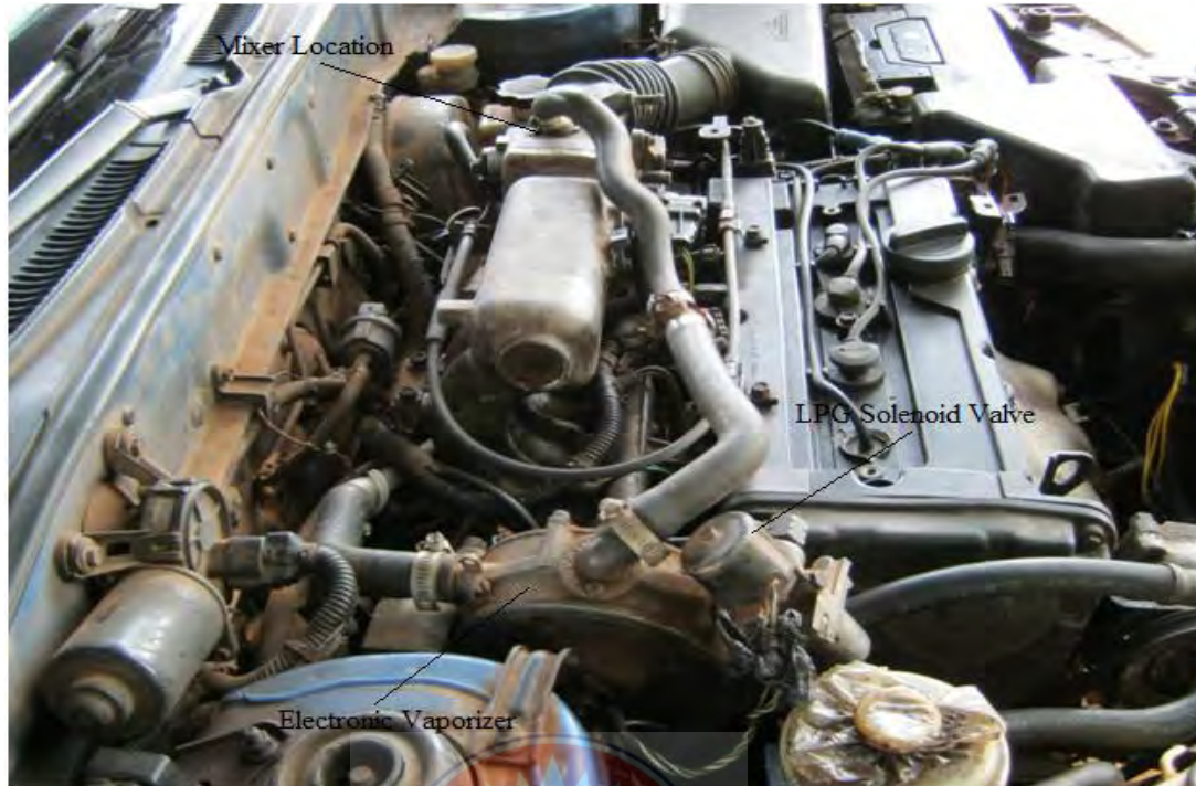
Figure 5.4. Fuel injection system; Using LPG and Petrol alternatively.
