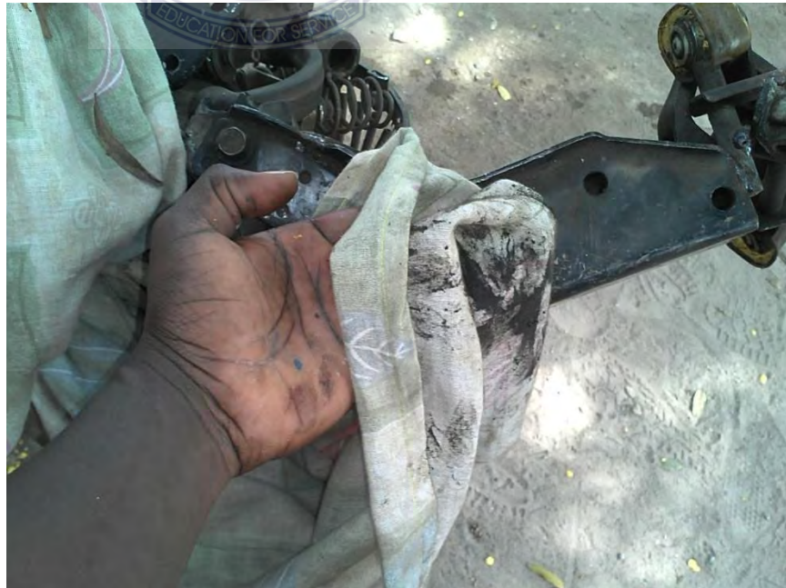
Figure 5.10: Preparing surfaces of scrap metals
