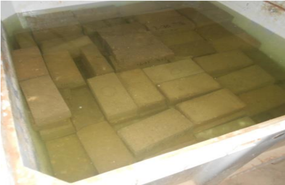
Plate 8: Specimens in water tank
