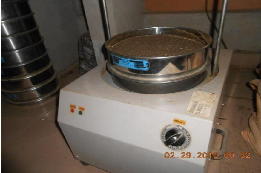
Plate 5: Sieving PKS on an electric shaker
