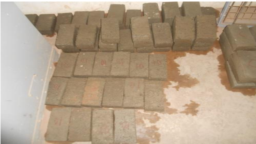
Plate 9: Specimens removed from tank after wet curing
