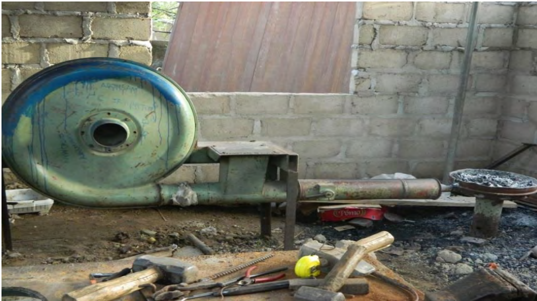
Plate 4.5: Manually powered blower for smelting
