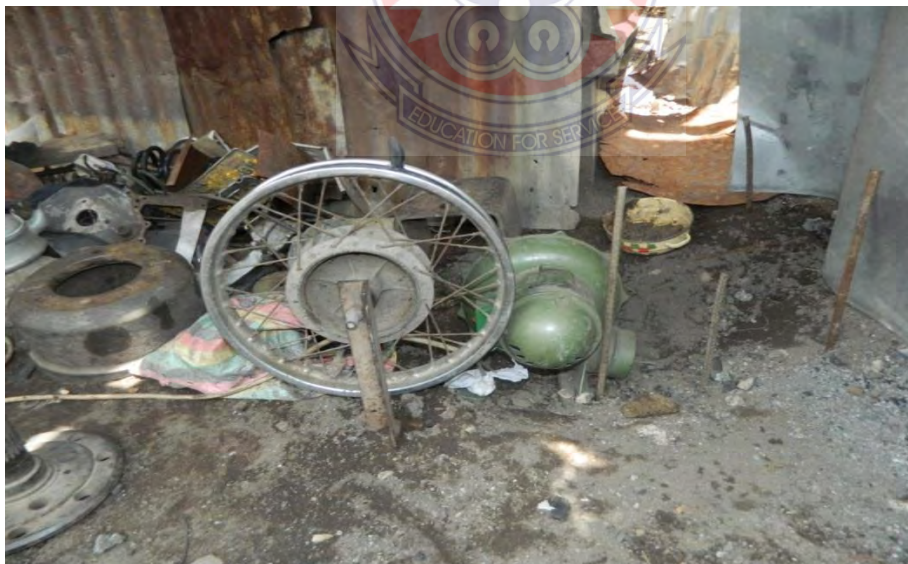
Plate 4.4: Electrically and manually powered blower for smelting
