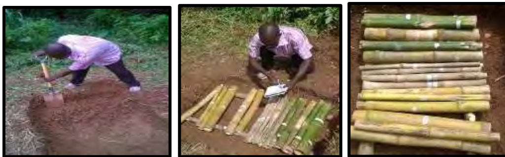
Figure 10.a: Carbonization of the Bamboo culms (preparation stage).
