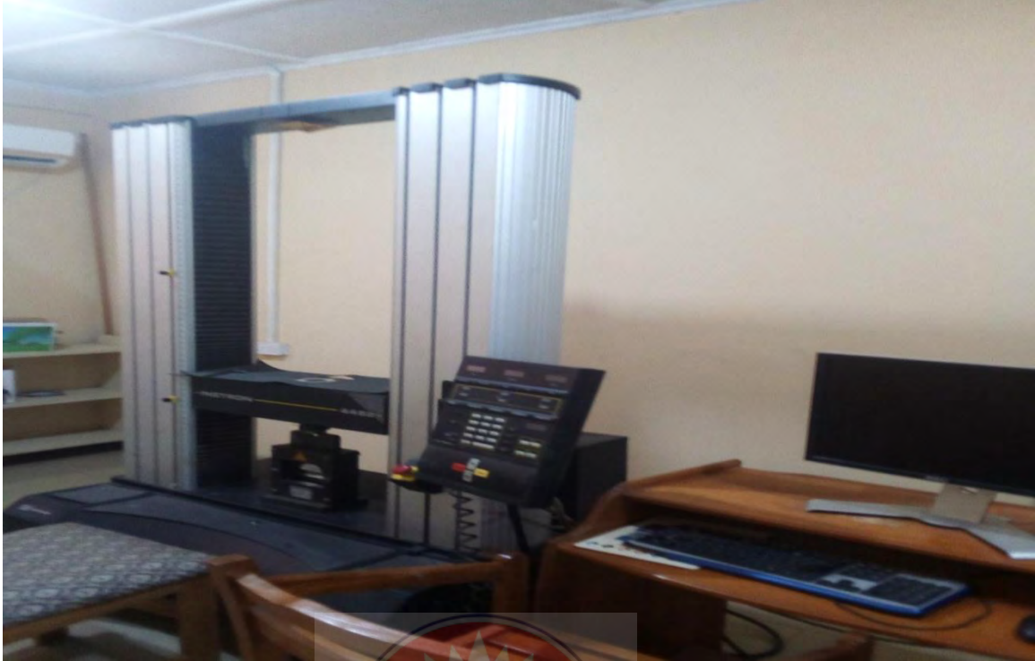
Figure 3.4. Shear strength test using Instron 4482 machine
