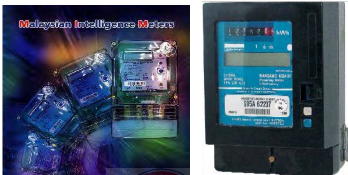
Figure 2.1: A smart Card Prepayment Metering System on Electronic Energy Meter
