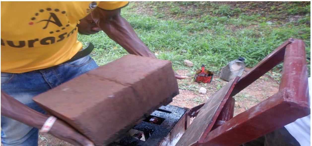
Figure 3.3 Removal of samples from the moulding machine
