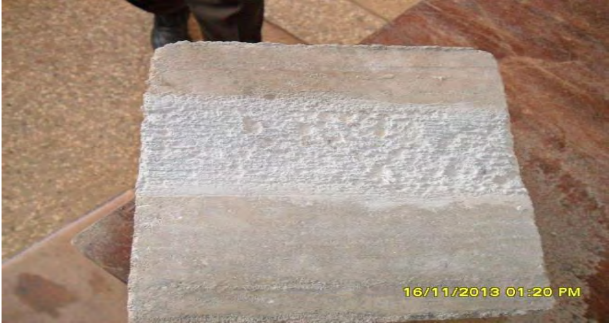
Figure 3.7: Sample cube after abrasion test
