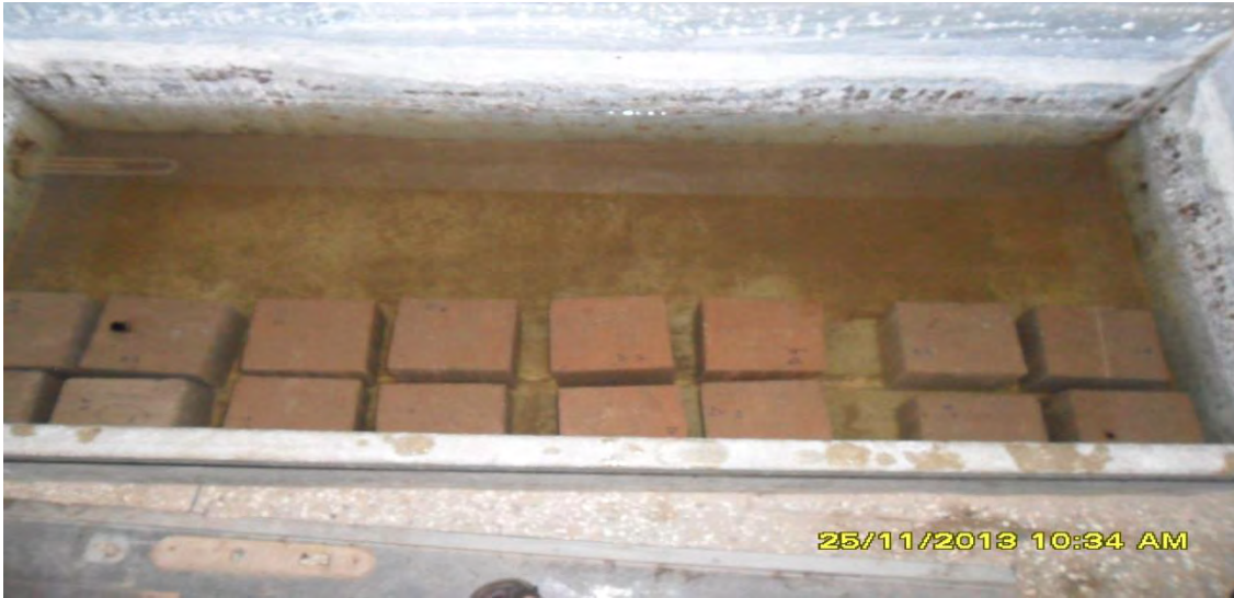
Figure 3.8: Conducting water absorption by total immersion.
