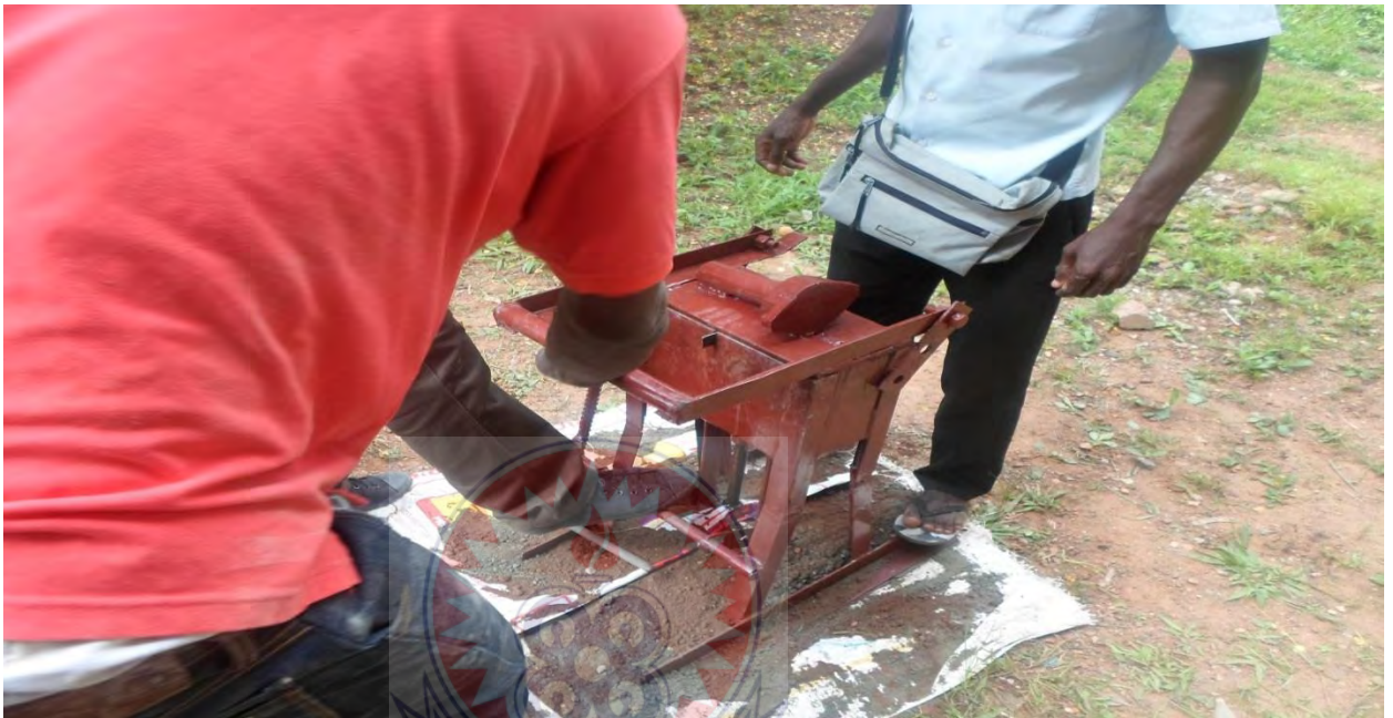
Figure 3.2 Tamping of samples
