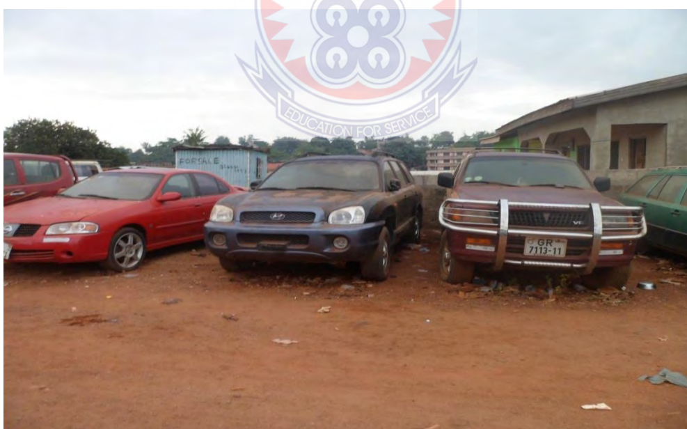
Plate 4.7: Damaged parts of these vehicles could not be replaced due to lack of spare parts
