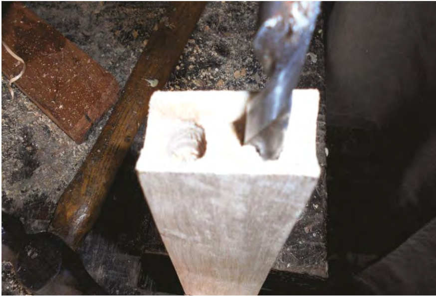
Figure 3.7 Drilling the end of side rails.
