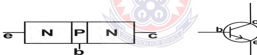
Figure 3.12a: block diagram of n-p-n transistor. Figure 3.12b: schematic diagram of n-p-n transistor.
