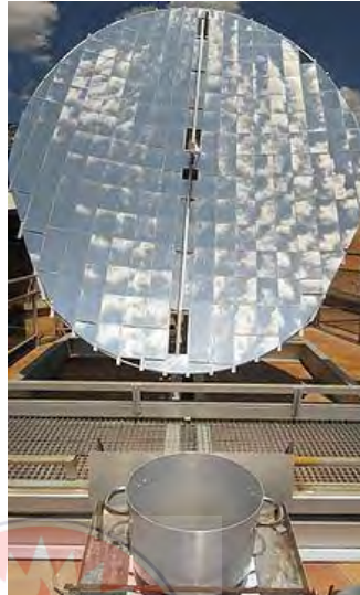
Figure 2. 7: A Scheffler cooker. This reflector has an area of 16 m 2 (170 sq ft), and concentrates 3 kW of heat
