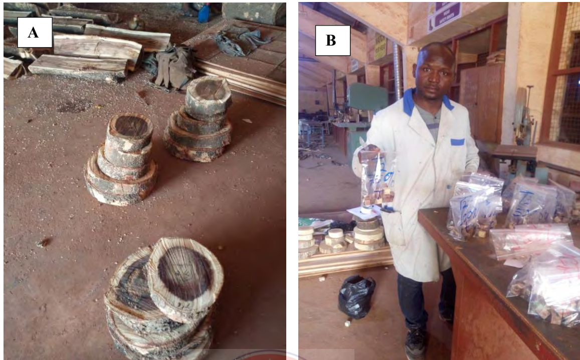
Figure 3.7: Discs Extracted From the Three Trees (A) and Sawn into Sizes (B)
