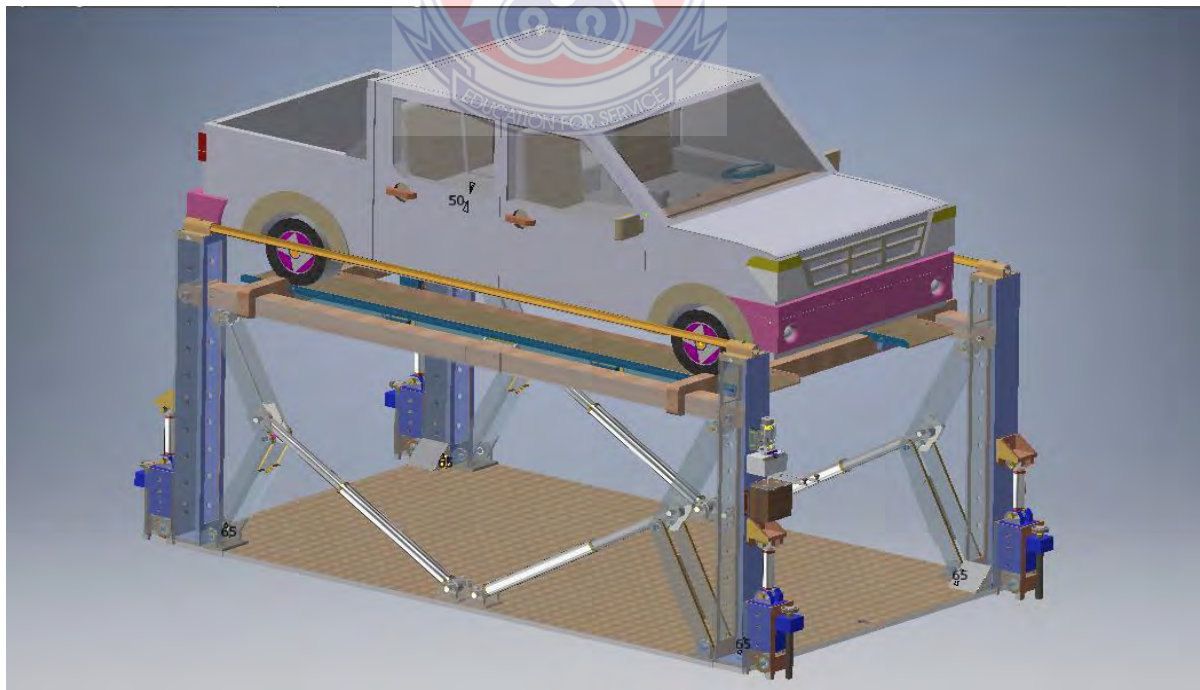
Figure 3.2, Model pick-up on new modified Lift at High Level
