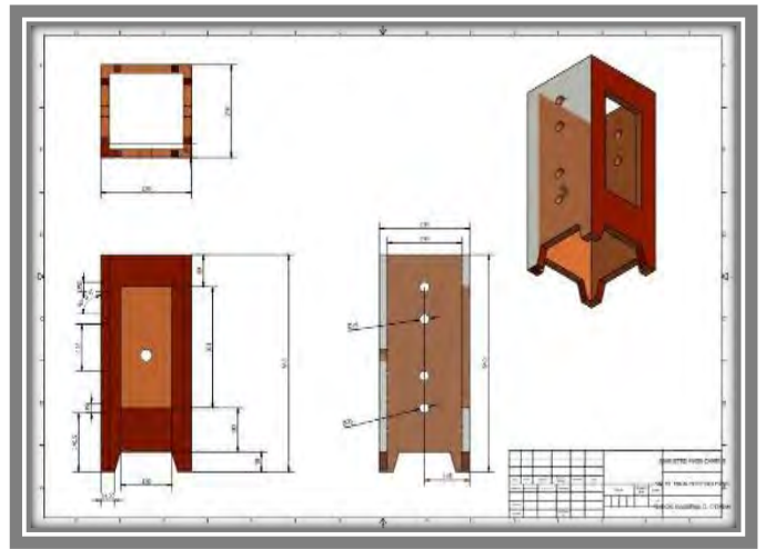
Figure 66, SN 39: Movable Wheel Main Post Operating Housing
