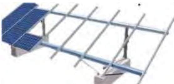
Figure 2.28: Ground mounting using concrete foundation
