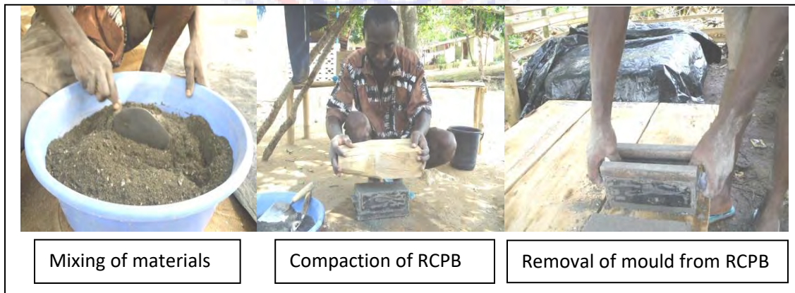
Figure 3.4: Preparation of RCPBs
