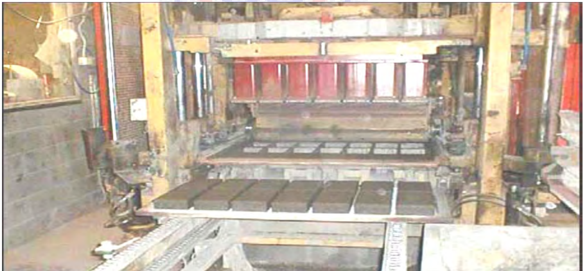
Figure 2.2: Tray of CPB moving out of compaction machine in factory (Holt and Raivio, 2005)
