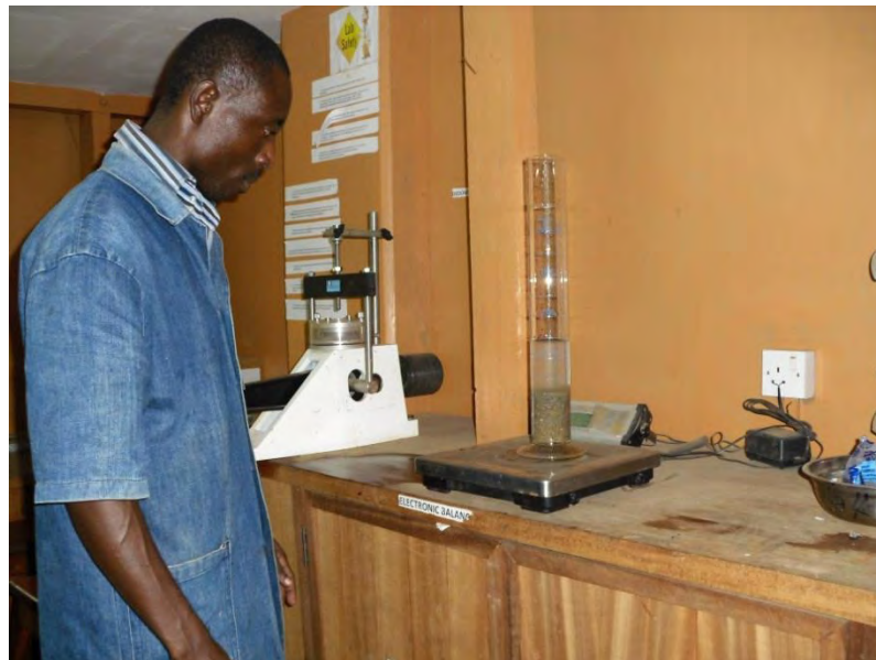
Figure 3.2: Taking the mass of flask filled with sand and water
