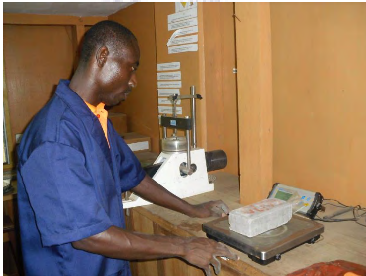
Figure 3.6: Weighing of RCPB
