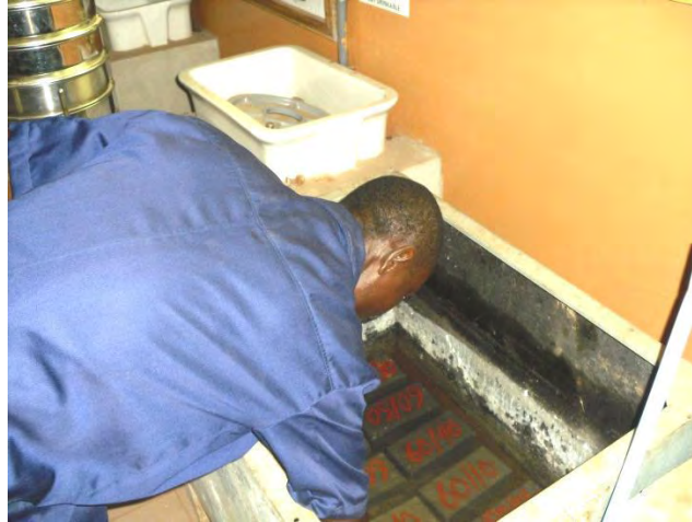
Figure 3.8: Immersion of specimens into tank containing water
