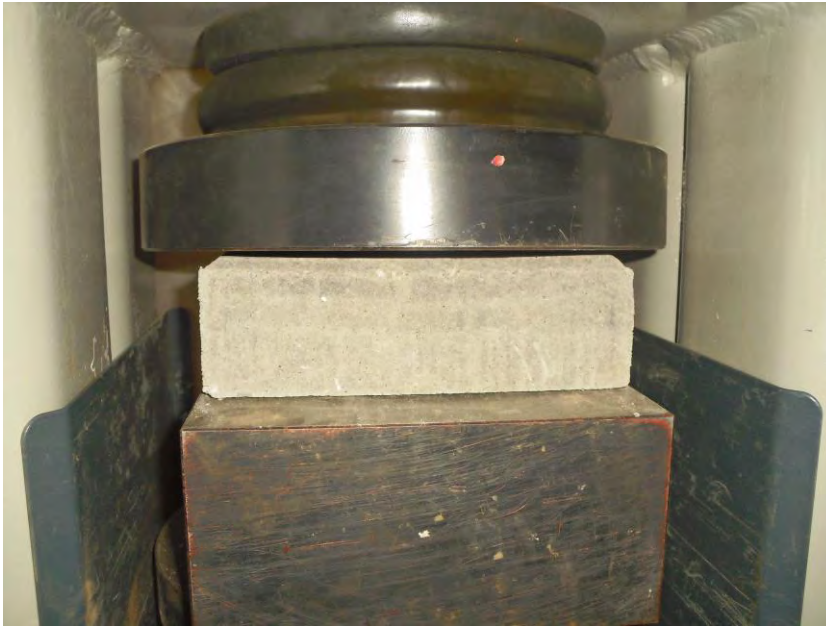
Figure 3.7: Set up of the compressive strength test
