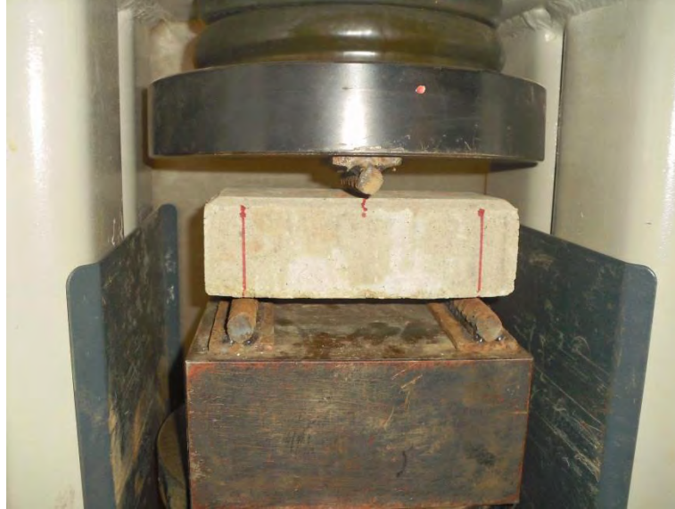
Figure 3.9: Set up of the flexural strength test
