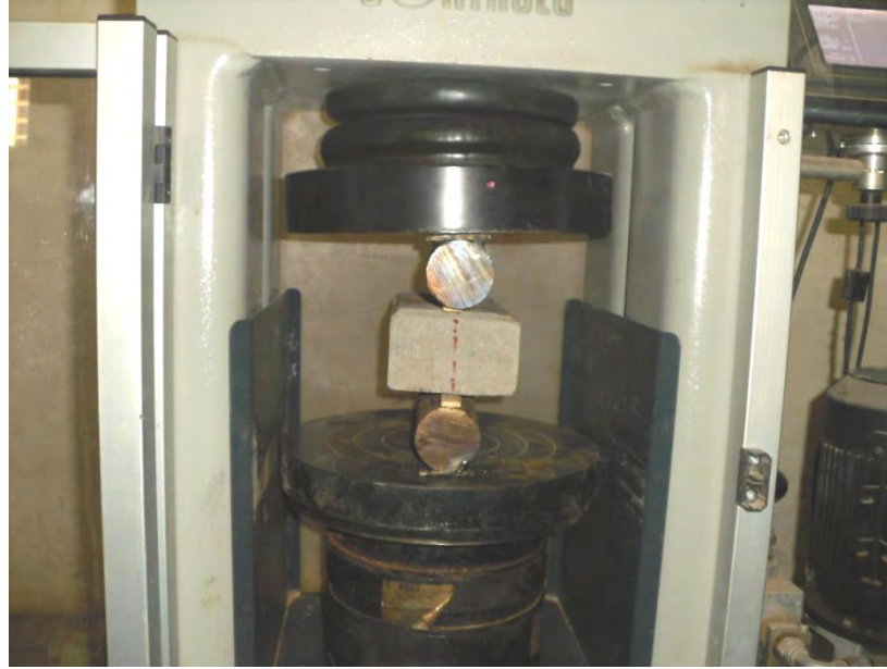
Figure 3.10: Set up of the splitting tensile strength test
