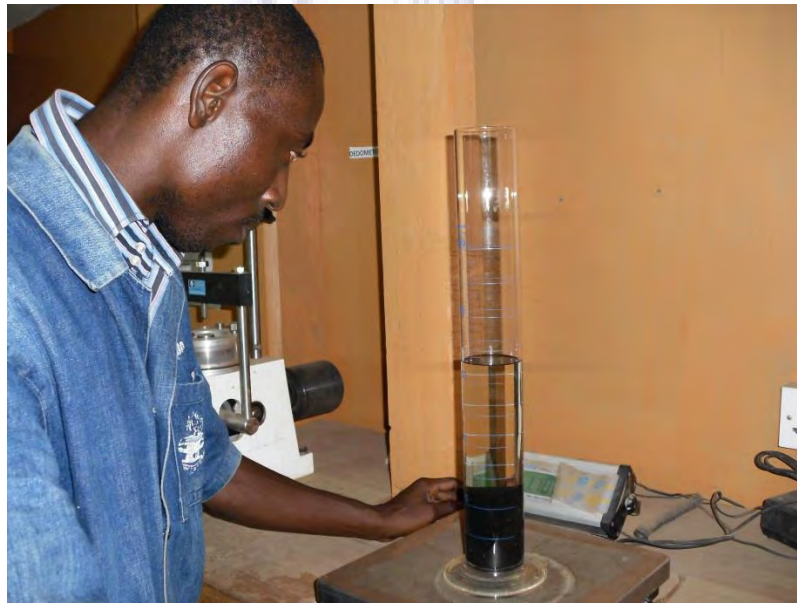
Figure 3.3: Taking the mass of flask filled with rubber and alcohol
