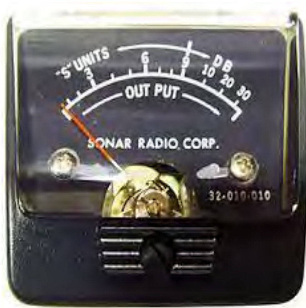
Figure 3.1: Photo Shot of the Signal Strength Meter Screen
