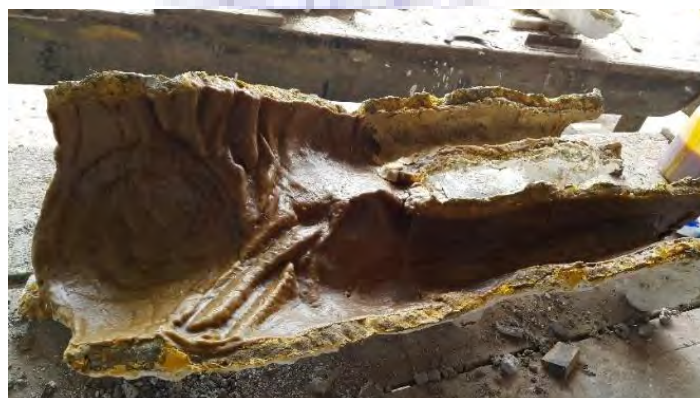
Figure 36: Wax Application onto the Mould
