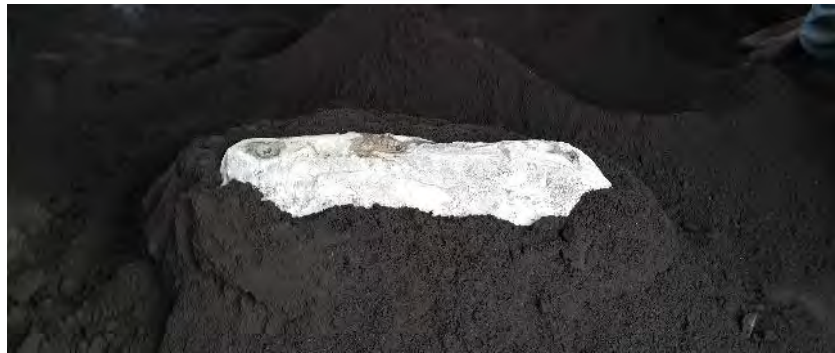
Figure 50: Mould Placed in the Sand
