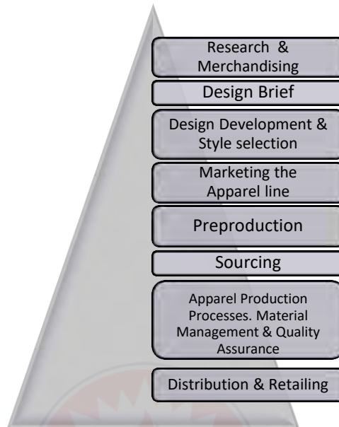
Figure 2.07: Eight-step generic commercial model for product manufacture.
