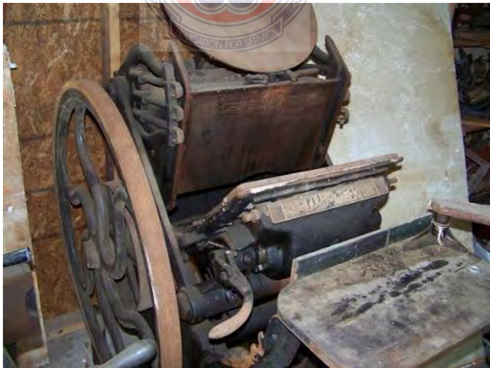
Figure 24. Jobber- Letterpress, Accra New Town (Source: field data, 2020)
