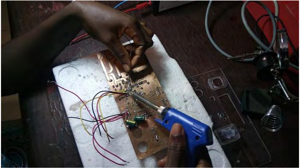
Fig. 3: Soldering of components on overboard.
