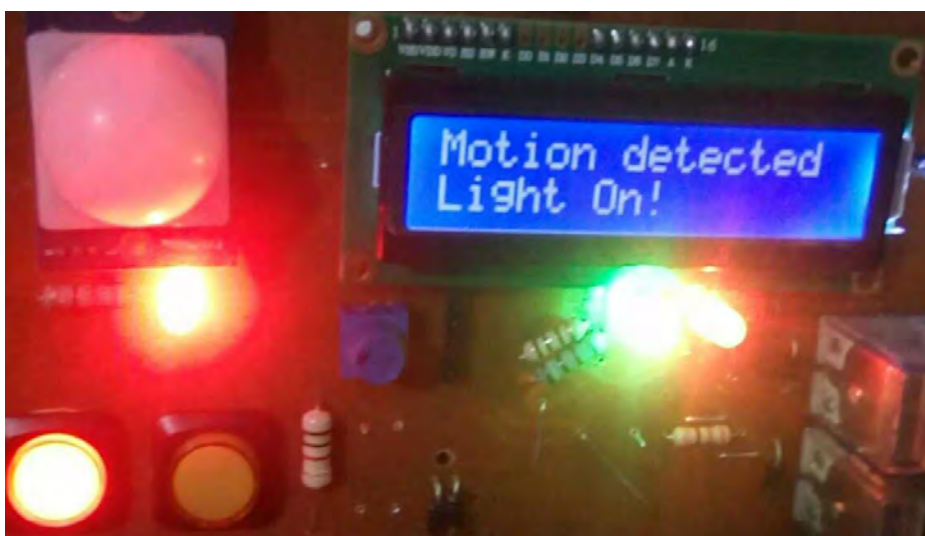
Fig. 4.6: Testing of device with light before assembly.
