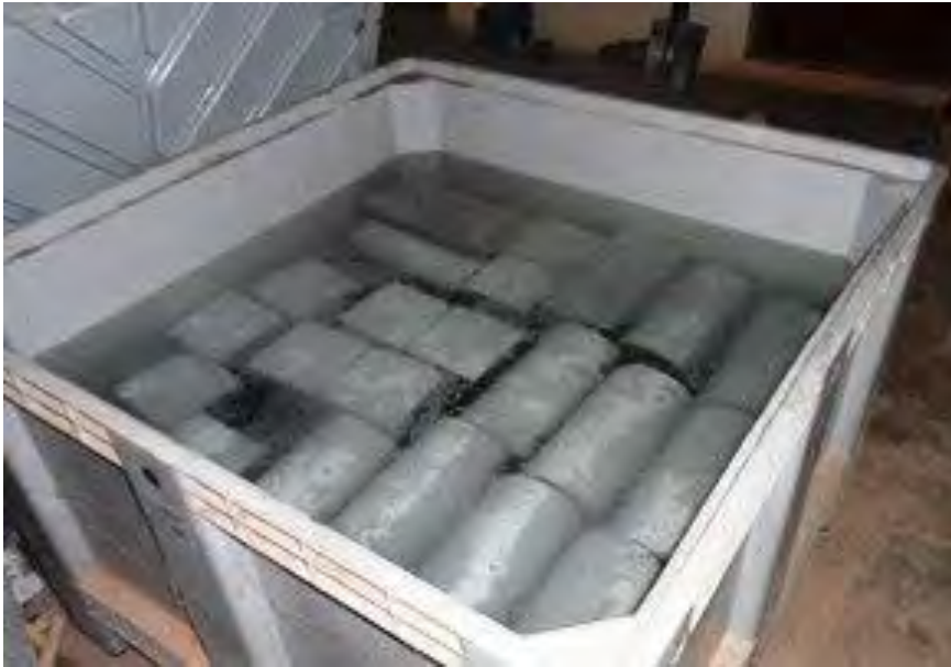
A7 Cubes and Cylinders Being Cured in Water
