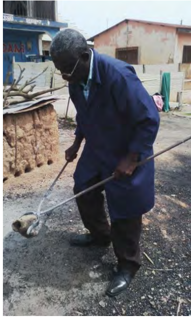
Fig. 20. & 21: Researcher and goldweight caster dewaxing moulds.
