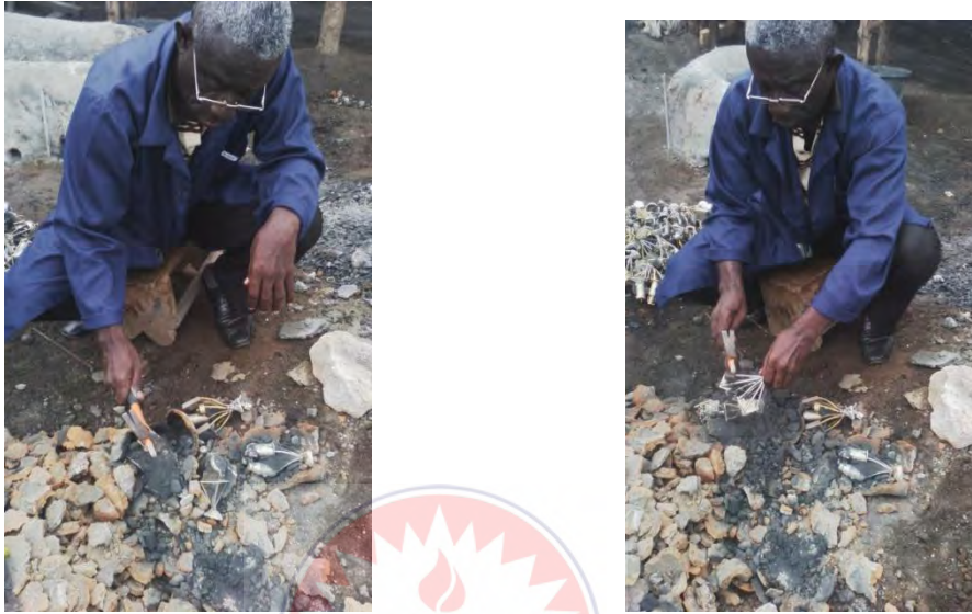
Fig. 26. & 27: Researcher breaking moulds to retrieve casting. Source: Field study (2017).
