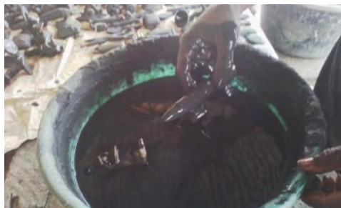
Fig. 16 & 17: Coating the wax models. Source: Field study (2017).
