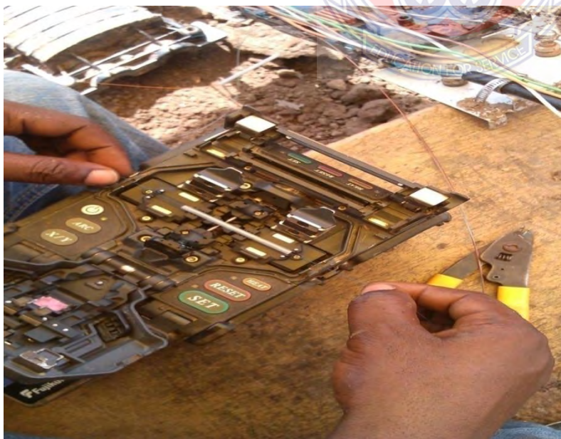
Figure 3: Splicing technique using the fusion splicer
