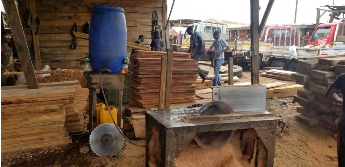
Plate 2.7 Circular saw in use virtually without any of the afore mentioned guidance
