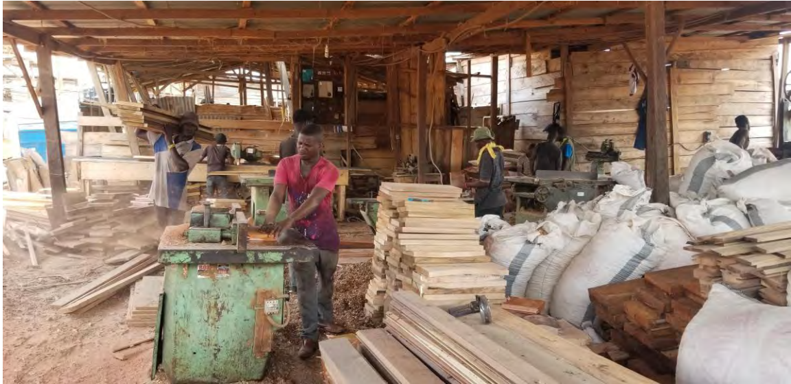
Plate 2a Spindle moulder operator without any of the safety gadgets in place neither on the machine or the user
