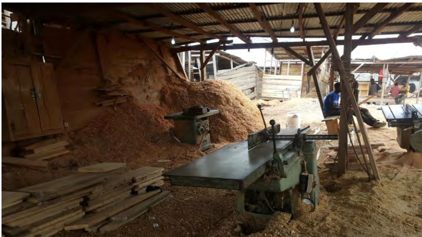
Plate 1.1 second-hand or used woodworking machines without the needed safety gadgets used in Kwadaso wood work machine shop.
