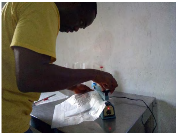
Figure 17: Using sealing machine to seal Polythene lining. Source: Working procedure by researcher.
