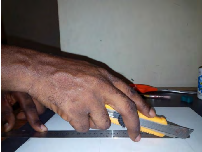
Figure 16: Scoring design along construction line.
