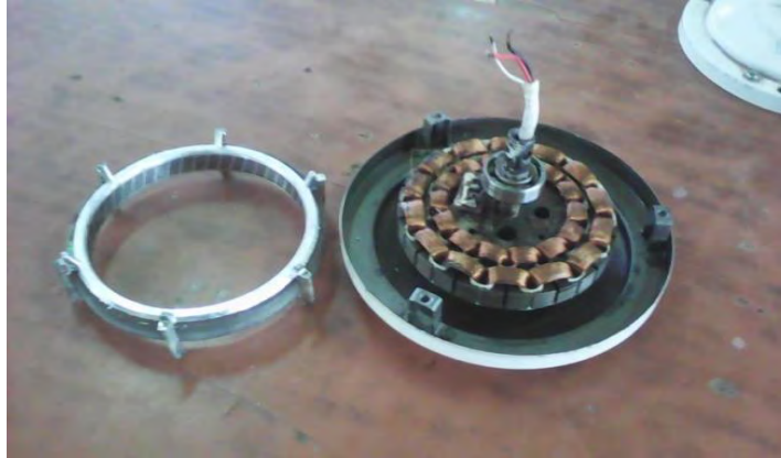
Figure 3.4: Shows a picture of fan with the armature and the capacitor removed to pave way for the magnet to be inserted.
