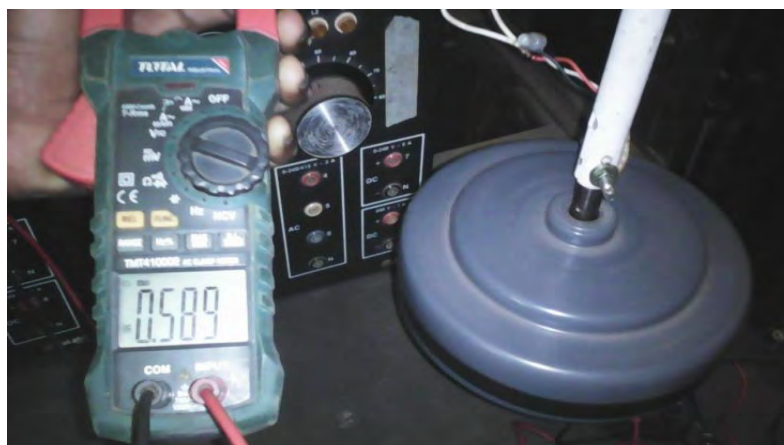
Figure 3.6: Shows a picture of the generator being re-assembled and tested using a multi meter to measure the current when the generator was put in rotation by hand.
