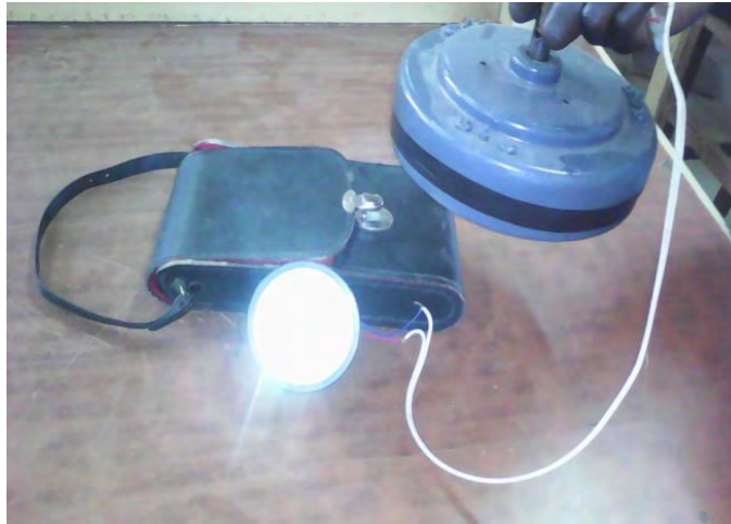
Figure 3.7: Shows LED lamp 'on', during testing.
