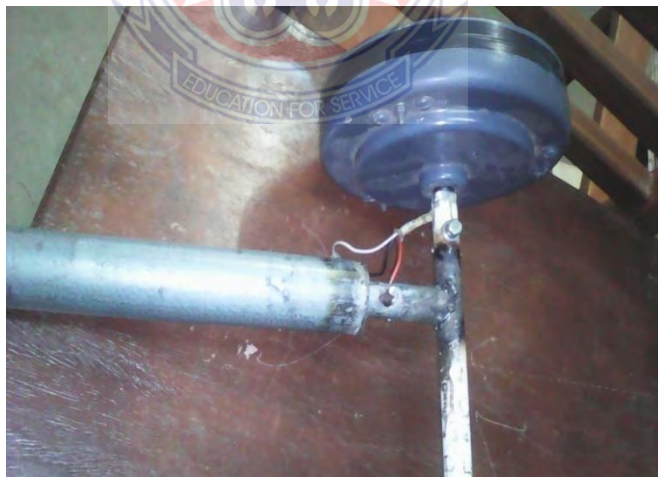
Figure 3.8: shows the generator connected to the yaw mechanism.
