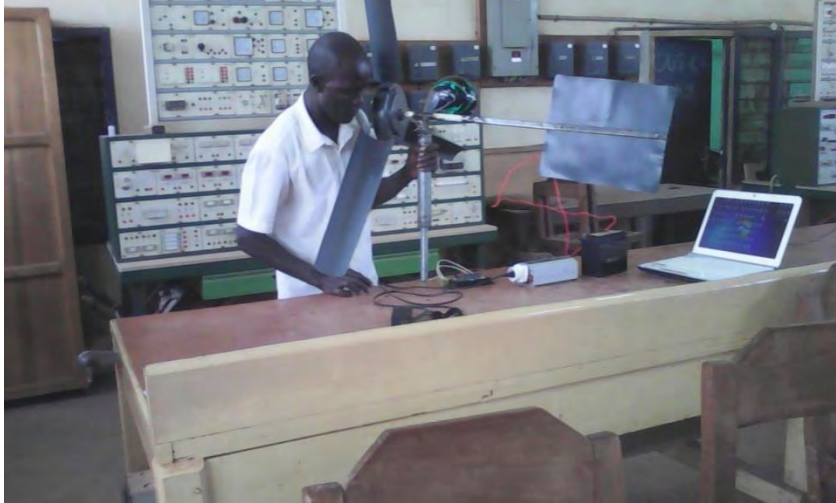
Figure 3.11: Shows the generator (wind turbine) connected to the electronic devices.
