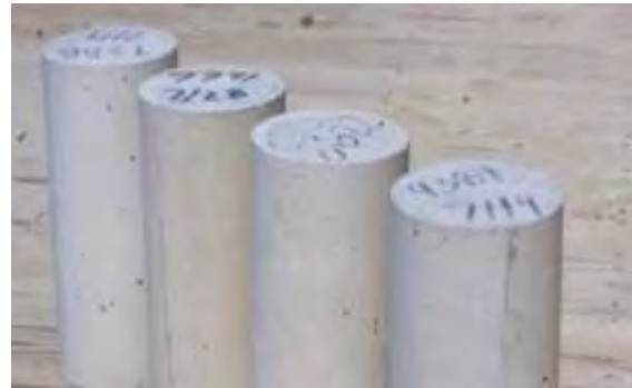
Figure 2.4 Concrete Cylinder Test
