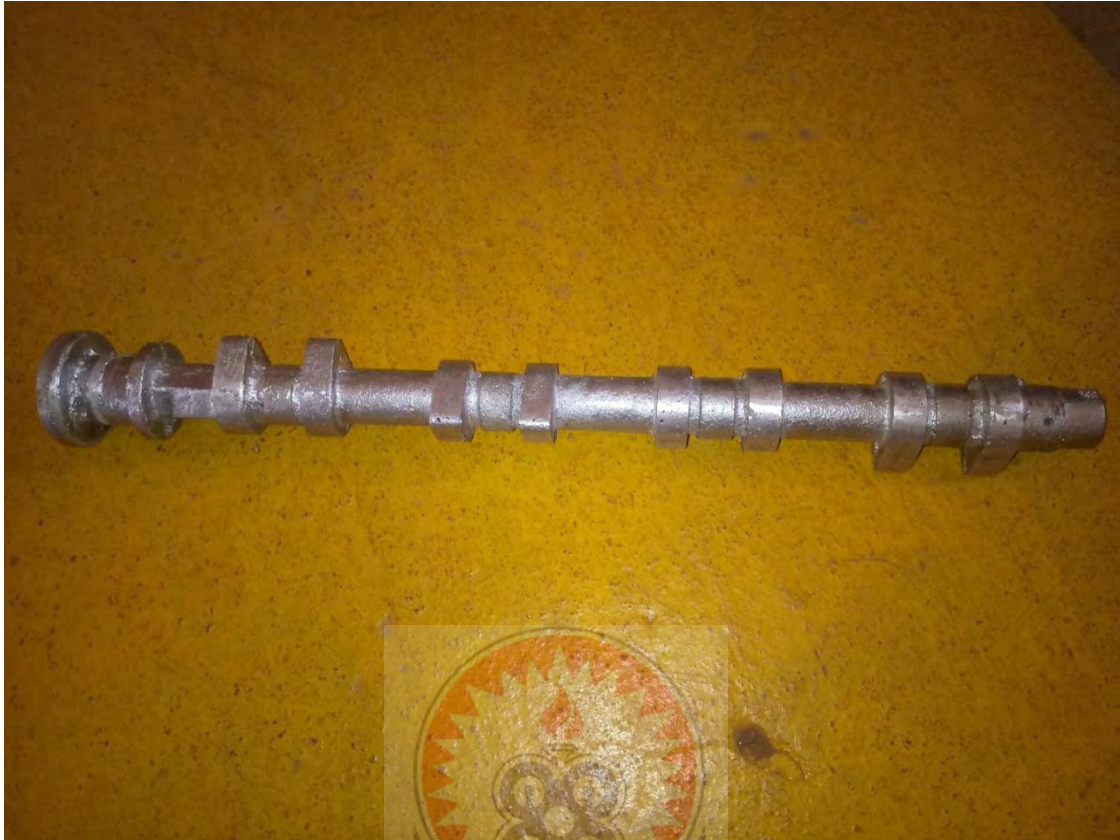
Figure 7: Cast Aluminium 6061 t6 Camshaft
