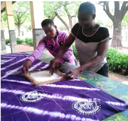
Plate 4.20- Step 1: Place the developed screen on the dyed fabric
