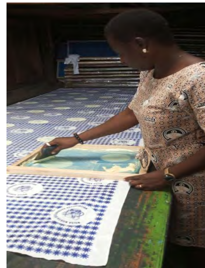
Plate 4.20- Step 1: Place the developed screen on the dyed fabric
