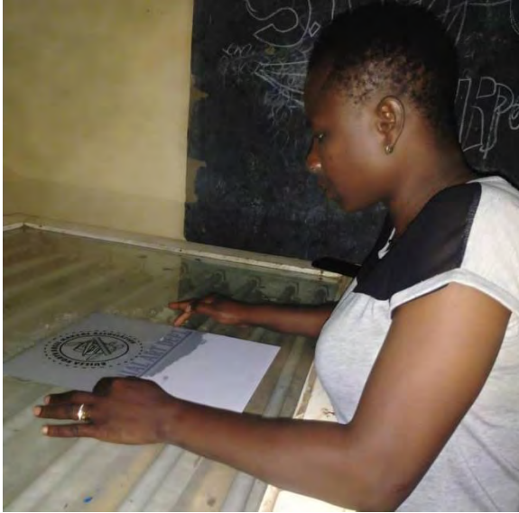
Plate 4.5 - Step 5: The coated screen was placed on the design.
