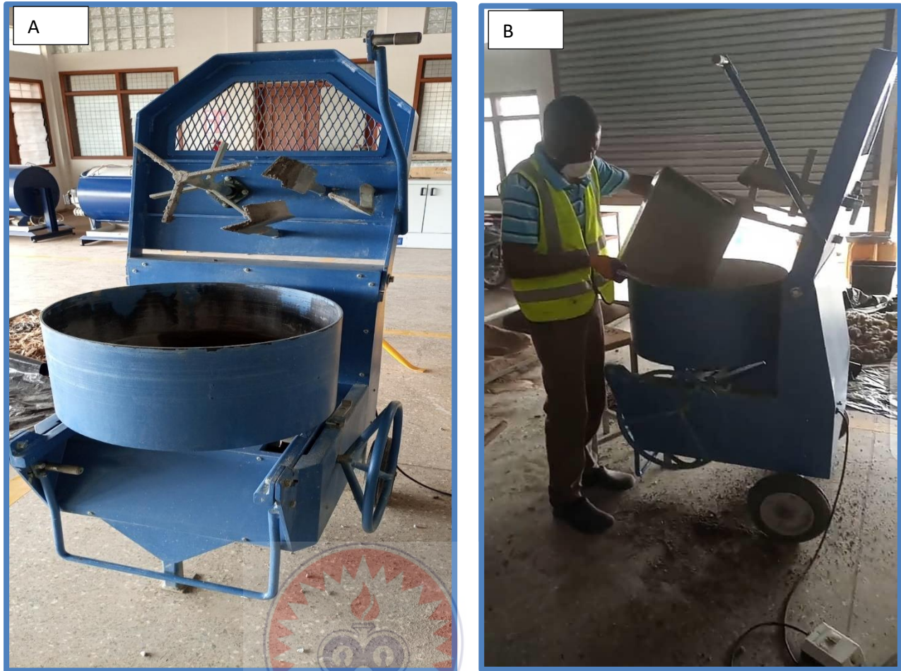
Figure 3.3 Pouring of the Measured Materials into the Pun Mixer
