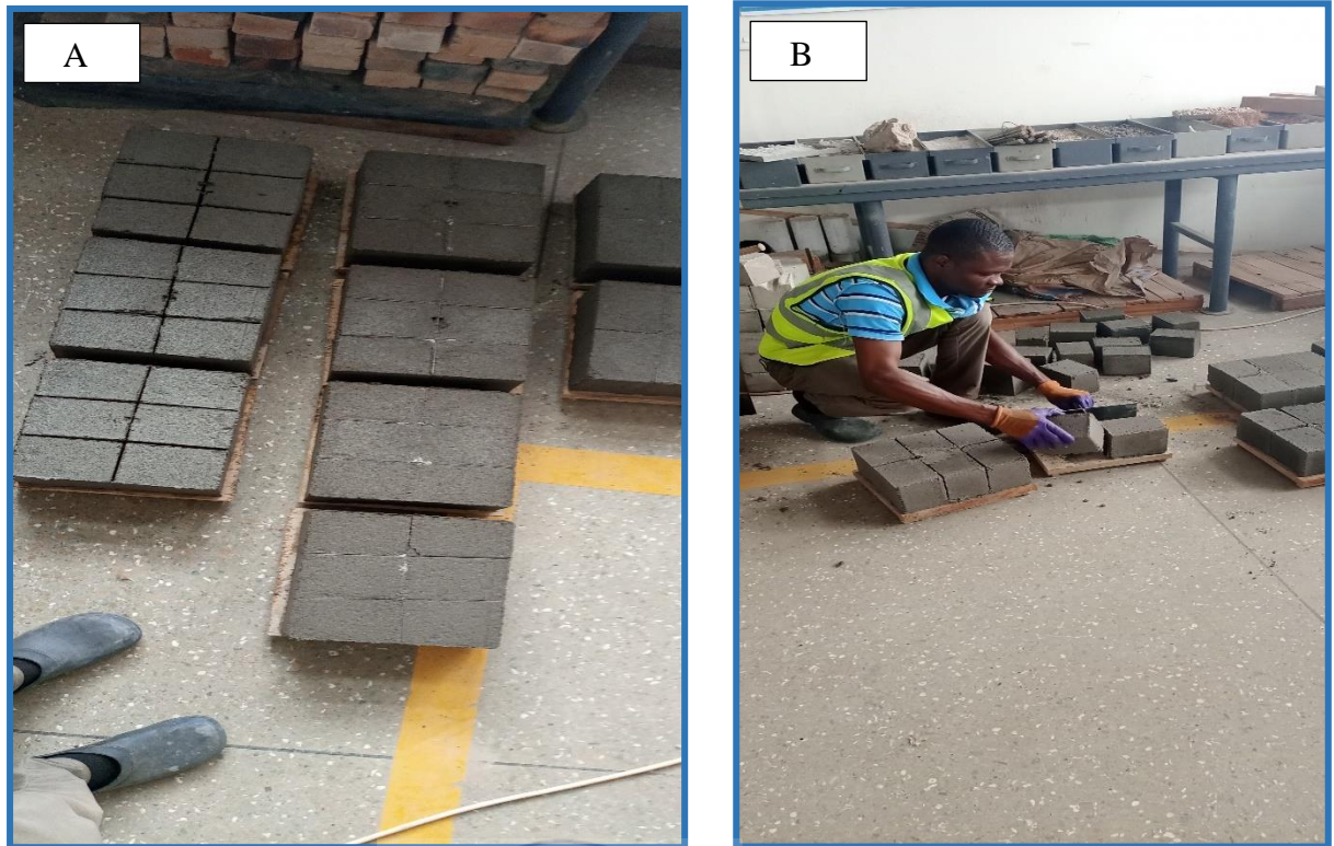
Figure 3.6 Storing of the Specimens on Wooden Pallets
