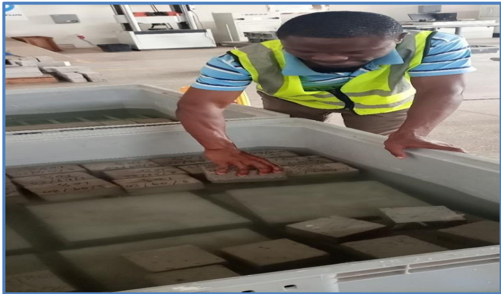
Figure 3.10 Specimens immersed in the water tank.
