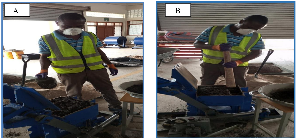
Figure 3.5 Pouring of the Mixture onto the Mould and Tamping the Mixture in Three Layers Using Wooden Tamping Rod.
