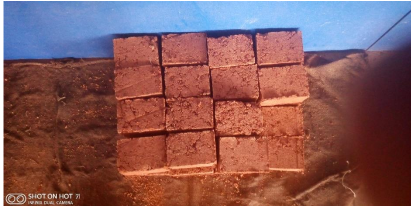
Figure 3.7 air-drying of the specimen
