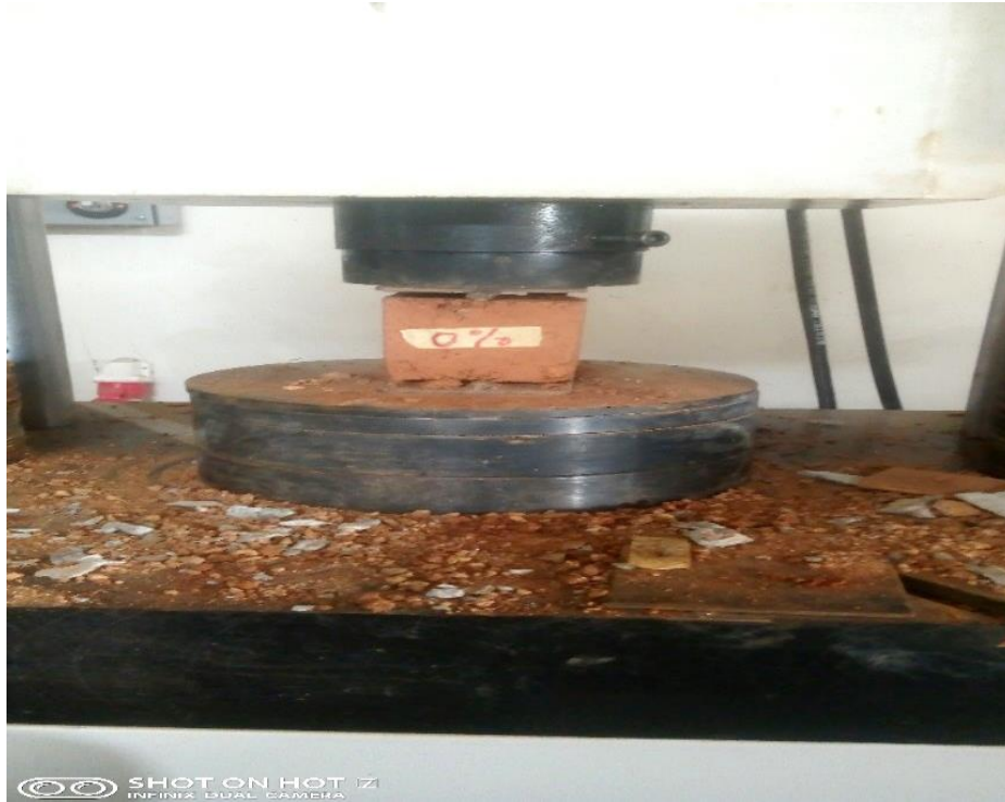
Figure 3.8: Centring of loading plate of the machine within the specimen.
