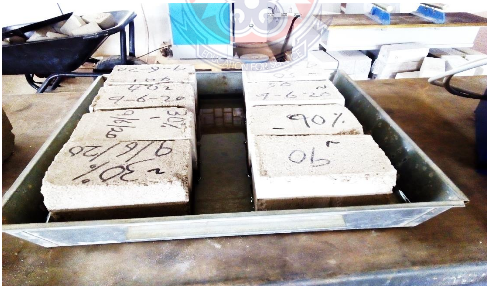
Figure 3. 12 specimens in water
