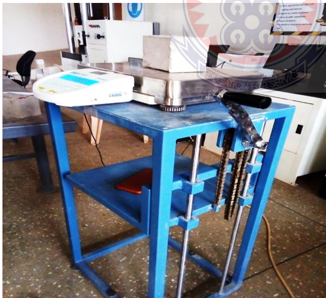
Figure 3. 13 Weighing of brick (electronic weighing scale,)
