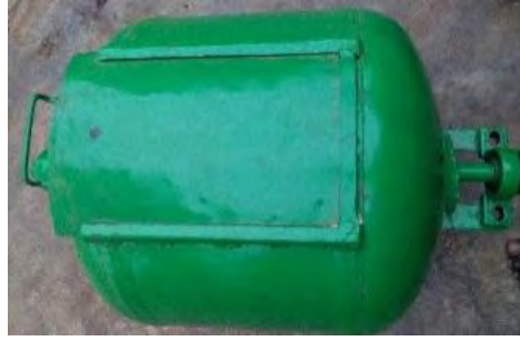
Figure 3.4: The Mixing Chamber
