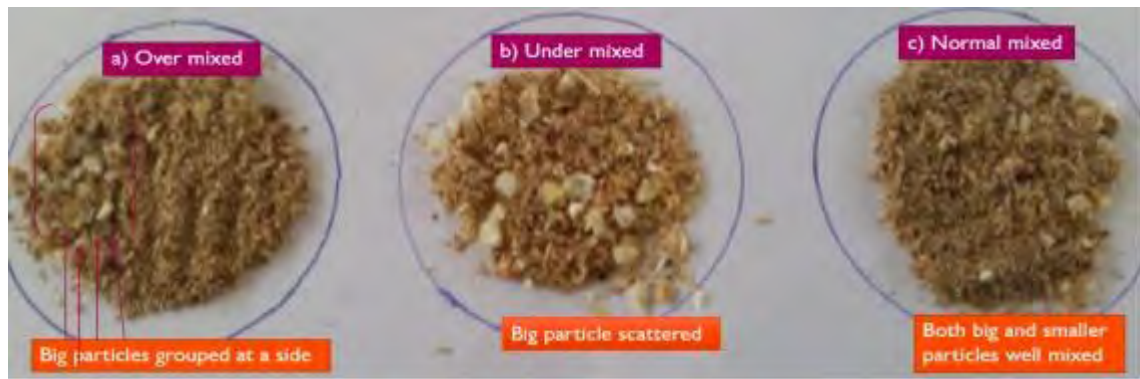
Figure 4.7: Mixed produce surfaces particle structure (a) Over mixed (b) Under mixed (c) Normal mixed .
