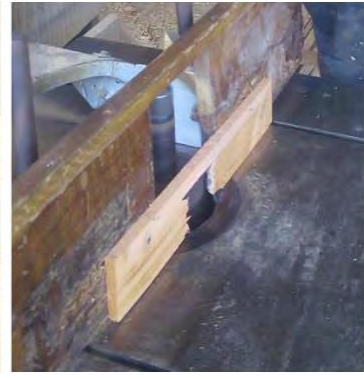
Figure 4.8: Spindle moulder without safety shield
