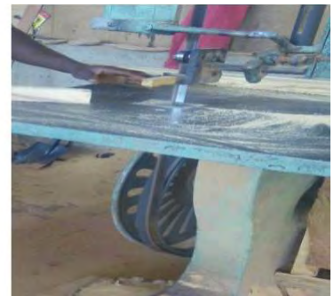
Figure 4.11: Bandsaw without enclosure of pulley mechanisms
