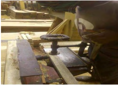
Figure 4.4: The wood mortise without any enclosure of safety bit and chuck
