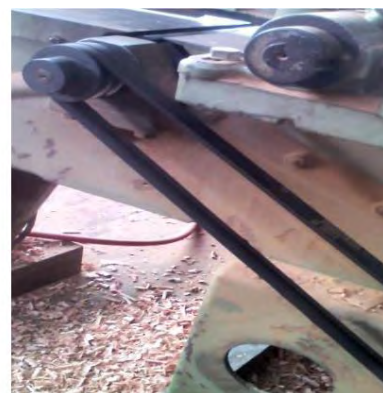
Figure 4.15 Surface planner without metal guard to enclose belt and pulley.
