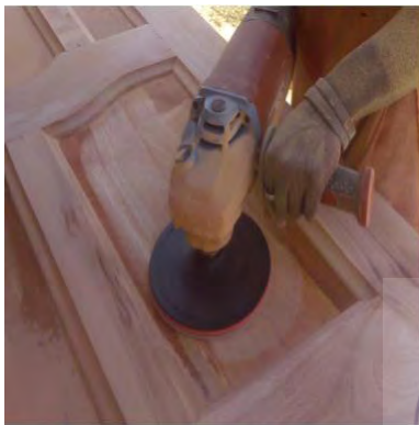
Figure 4.12: Sander without guard to enclose drum and disc
