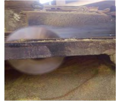
Figure 4.18: Circular saw without a blade guard
