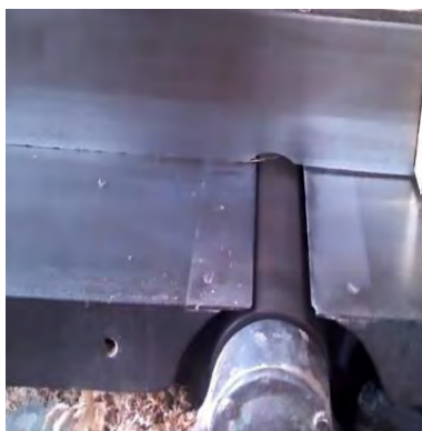
Figure 4.14: Surface planner without cutter head guard.
