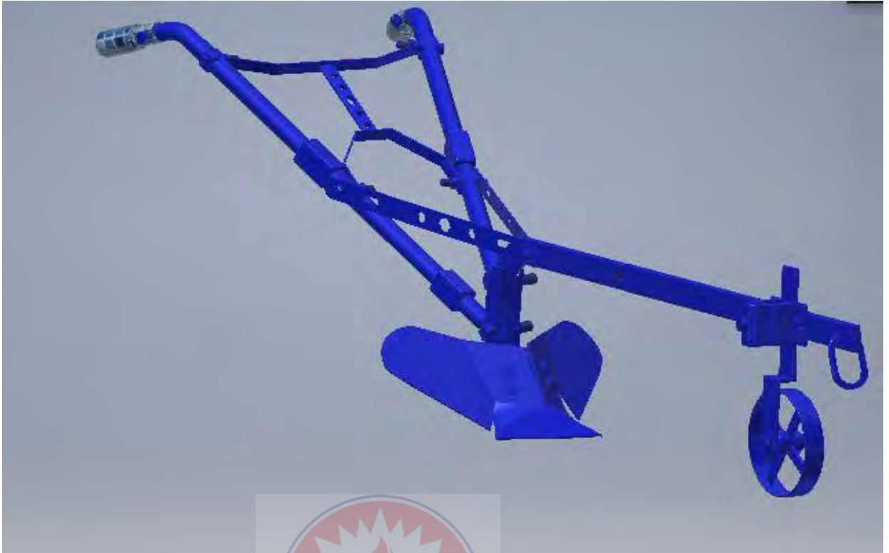
Figure 3.4. Assembled Mouldboard Plough
