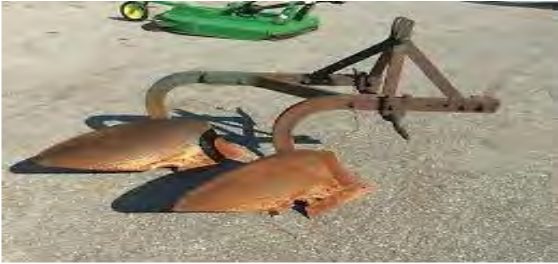
Figure 2.9. Broken Mouldboard Plough
