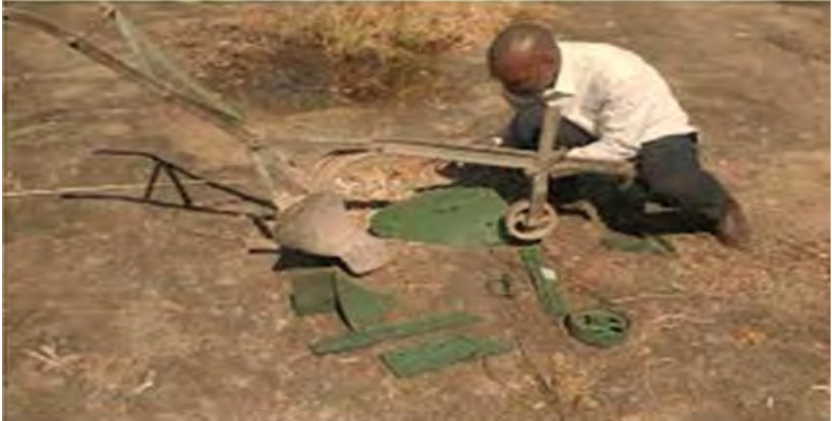
Figure 2.10. Replacement of Some Broken Parts of a Mouldboard Plough
