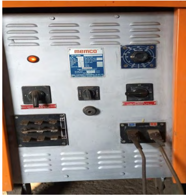
Figure 3.8 Welding Machine (KNUST Workshop, 2020)
