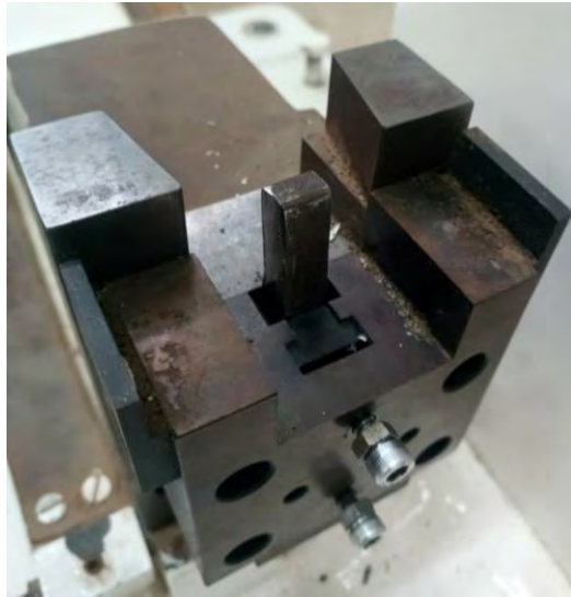
Figure 3.14 Specimen in Impact testing machine
