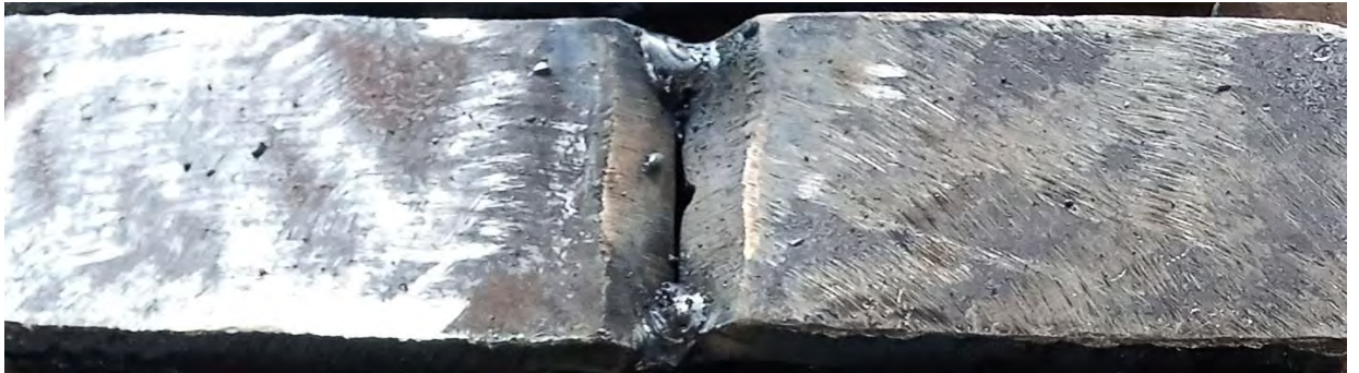
Figure 3.3 Set-up of tacked weld
