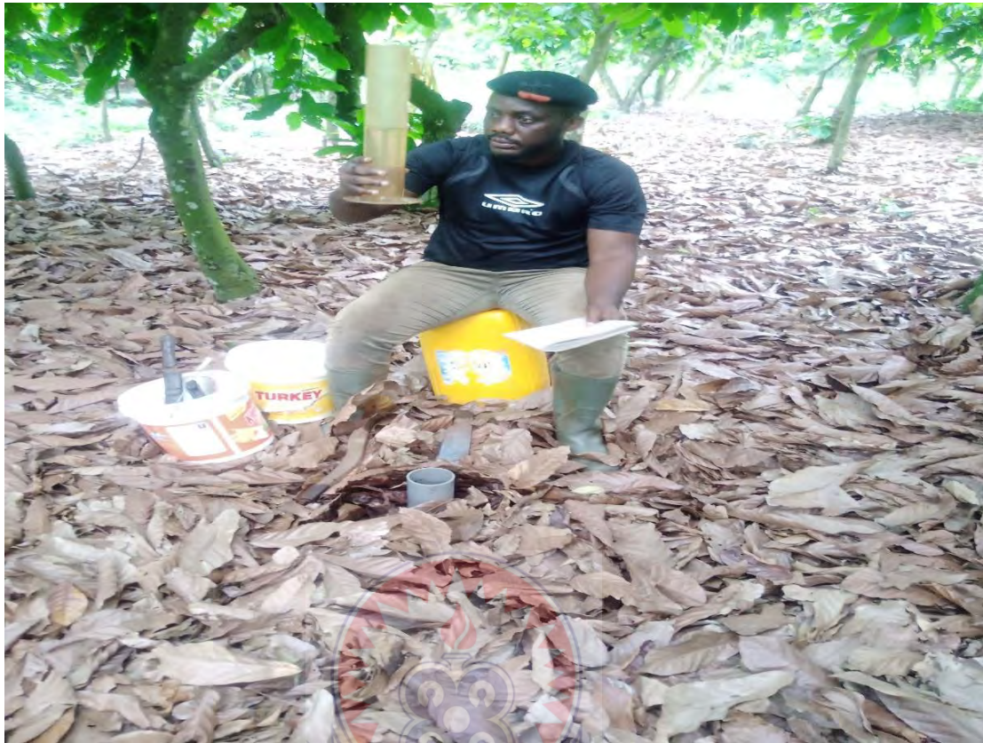
Plate 3.7 Researcher measuring infiltration amount using the single ring method
