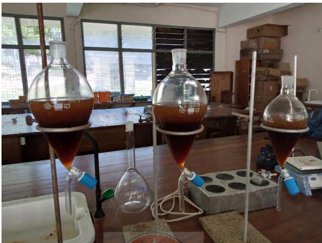
Figure 11: Using separating funnel to collect the ethyl acetate layer from the aqueous layer.
