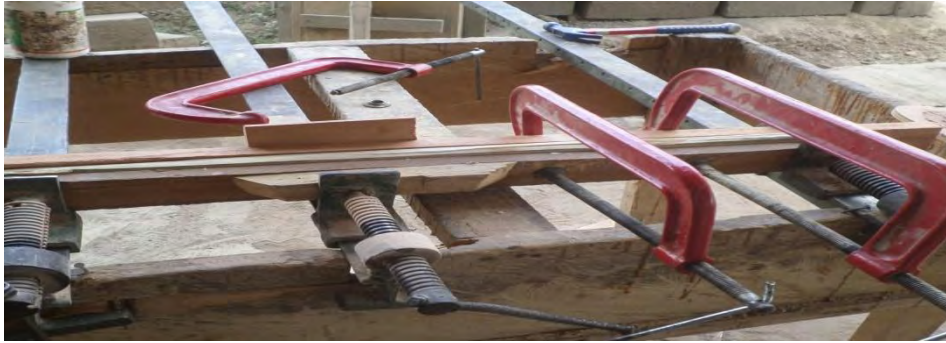
Figure 3.9: Picture of glued Bambusa vulgaris strips in clamps
