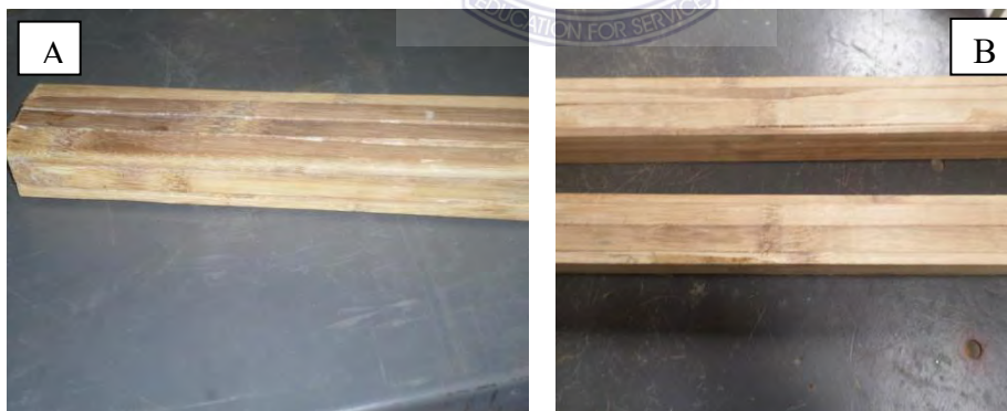
Figure 3.10: Sample of laminated bamboo: sample „A“ for mature and sample „B“ for juvenile.
