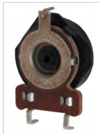
Fig. 2.7: potentiometer for adjusting the ultrasound frequency
