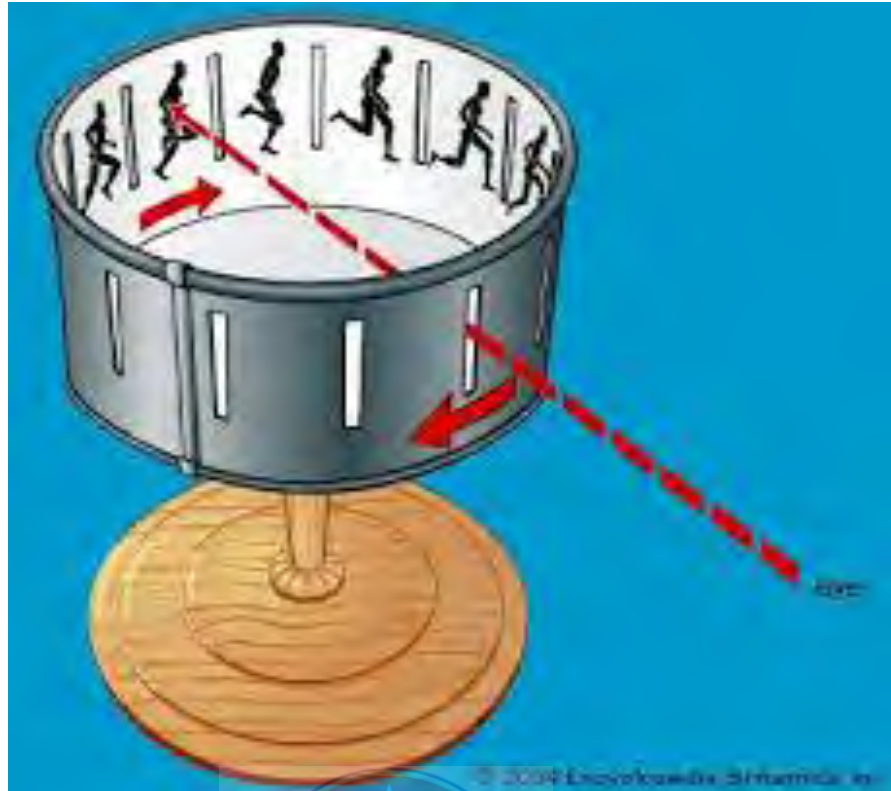
Fig 5: Zoetrope; motion-picture device https://www.britannica.com/topic/dice
