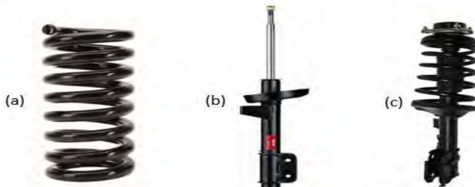
Figure 2.5: Types of coil springs (a) Coil spring (b) Strut (c) Pre-assembled unit
