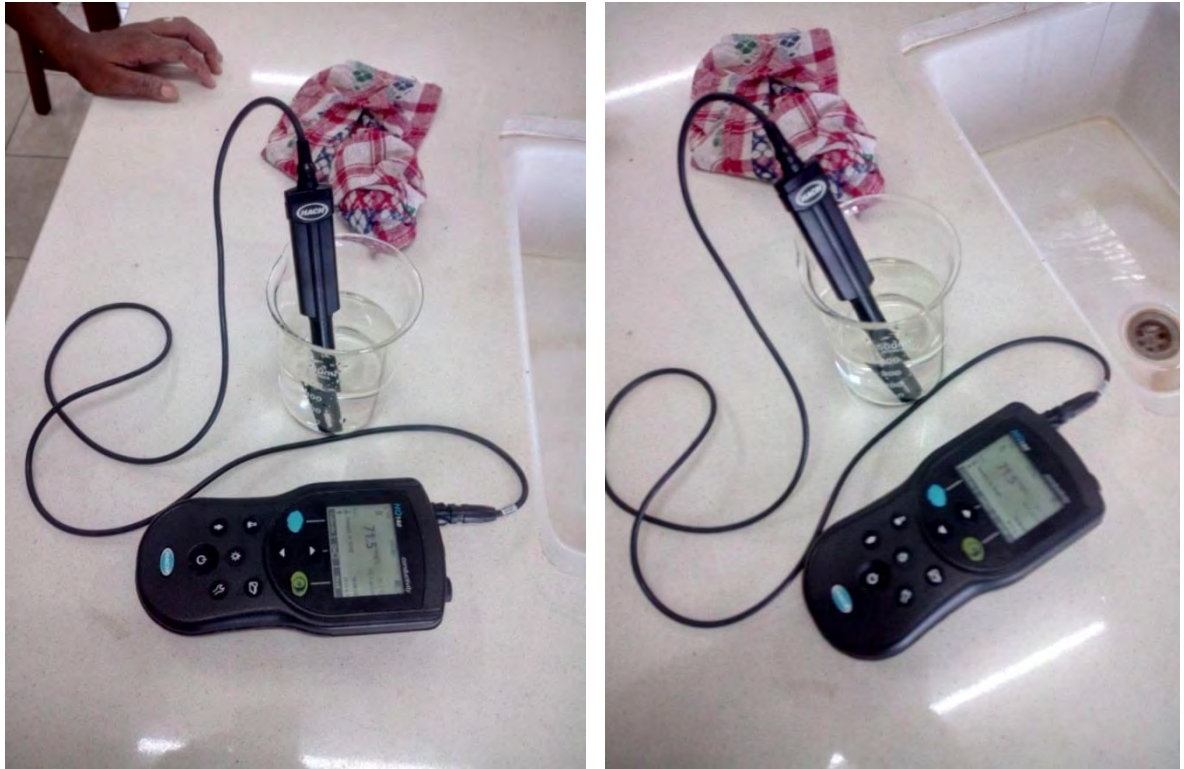
Figure 3.11: Electrical conductivity taken from sample water
