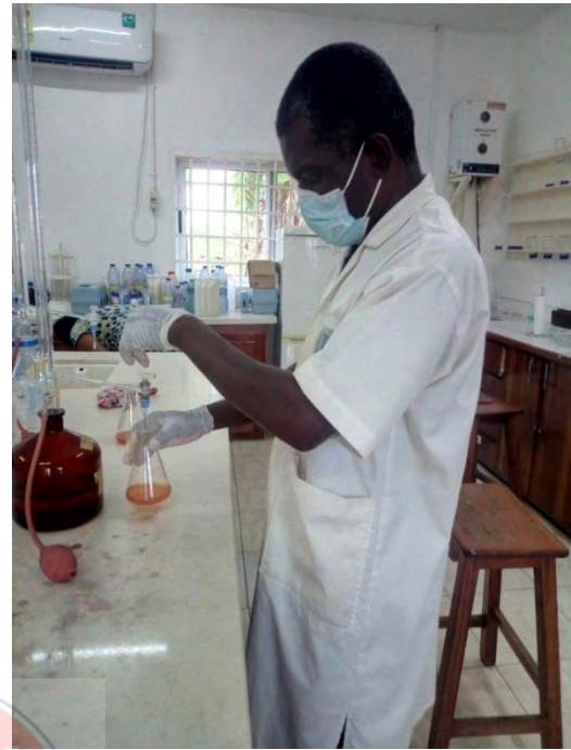
Figure 3.17: Researcher using titrating for chloride
