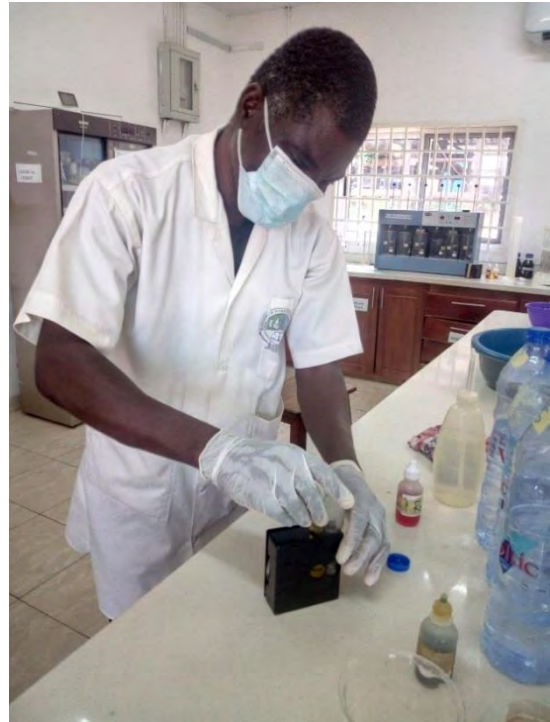
Figure 3.12: Colourimeter being used to take pH of sample water
