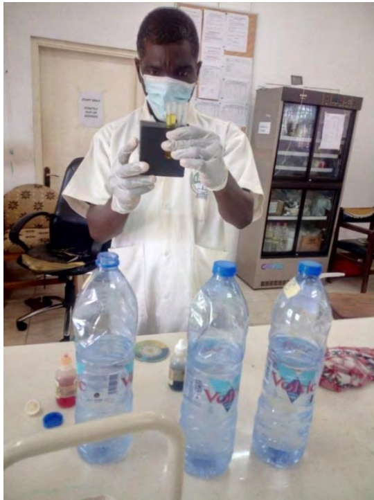
Figure 3.12: Colourimeter being used to take pH of sample water
