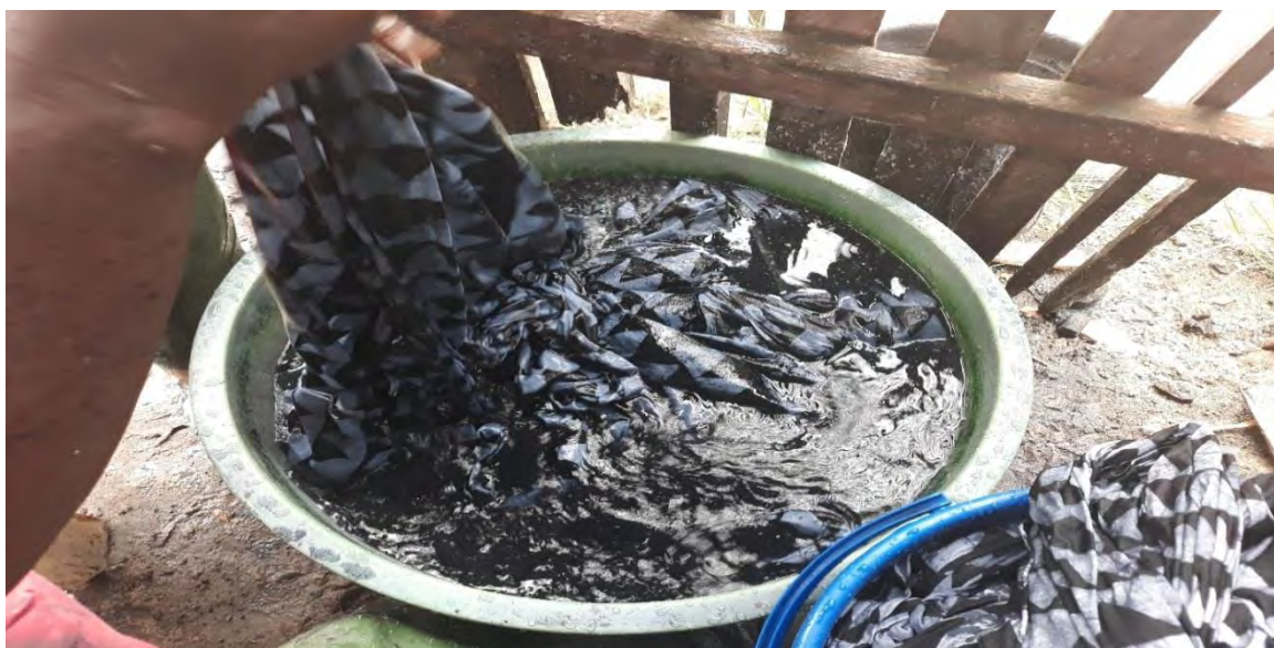
Figure 15: Rinsing of fabric after washing (Source: Fieldwork, Data, 2019, Cape Coast )
