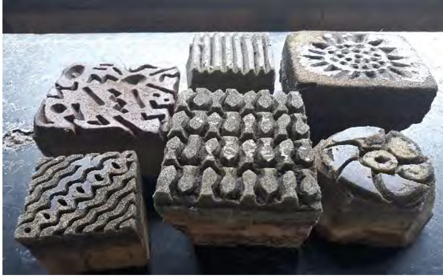
Figure 5: Designed Foam blocks for application of wax
