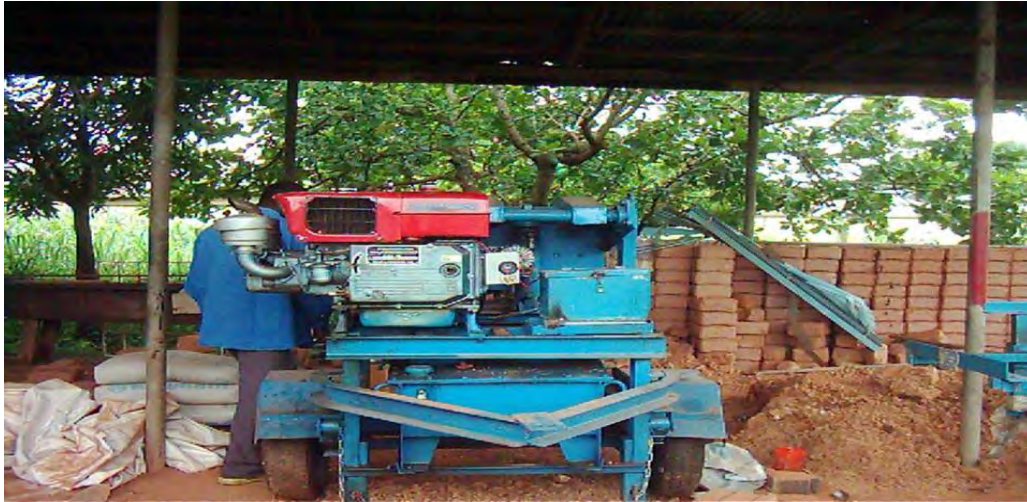
Fig2.4Hydraulic Machine developed for hydrafoam block moulding.
