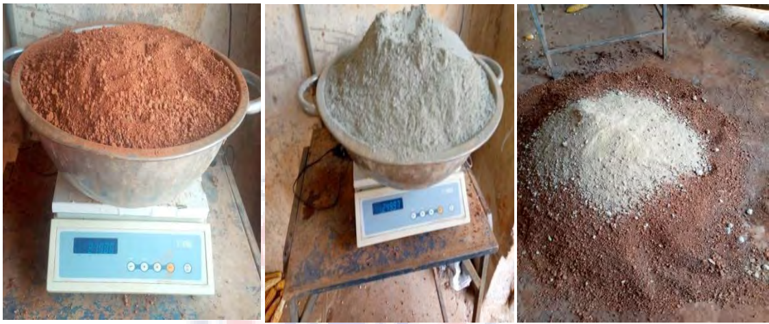
Figure 3.6: batching of the various percentages of the materials.
