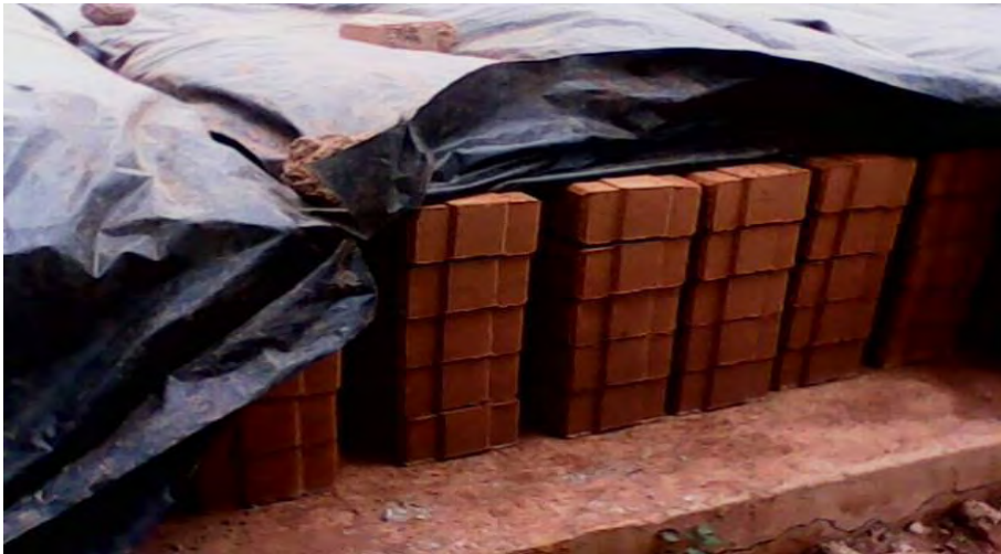
Figure 3.8: Curing of the specimen with water and polythene sheets, for 28days
