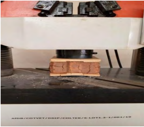
Figure 3.9.1: Stress-strain test set up.
