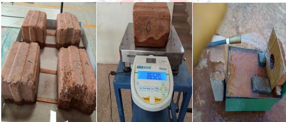
How water absorption (left) density (middle) and erosion (right) tests were conducted
