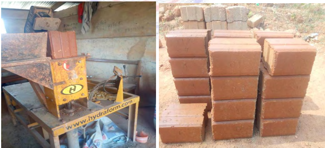
Figure 3.7: Hydraform interlocking blocks machine with single mould and blocks
