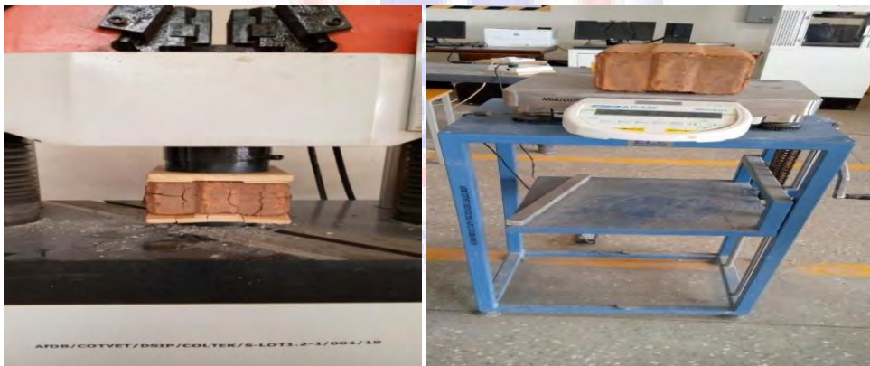
Figure 3.9: Compressive Strength test set up
