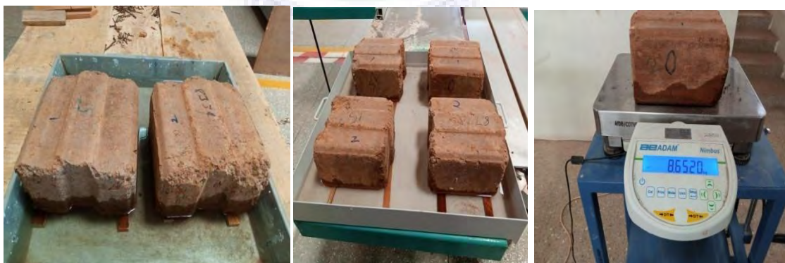
Figure 3.11: Water Absorption Test Procedure
