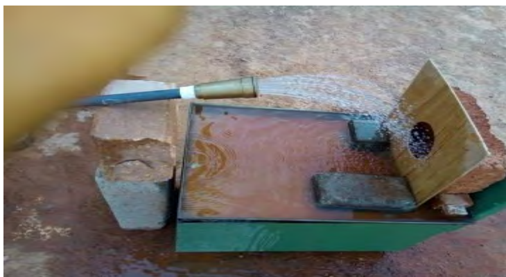
Figure 3.12: Erosion Test set Procedure
