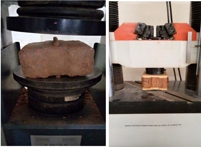
How tensile (left) and compressive (right) tests were done in the laboratory
