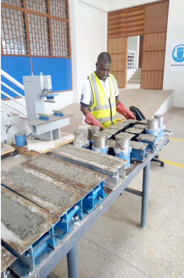
Casted Concrete Cubes and Beams
